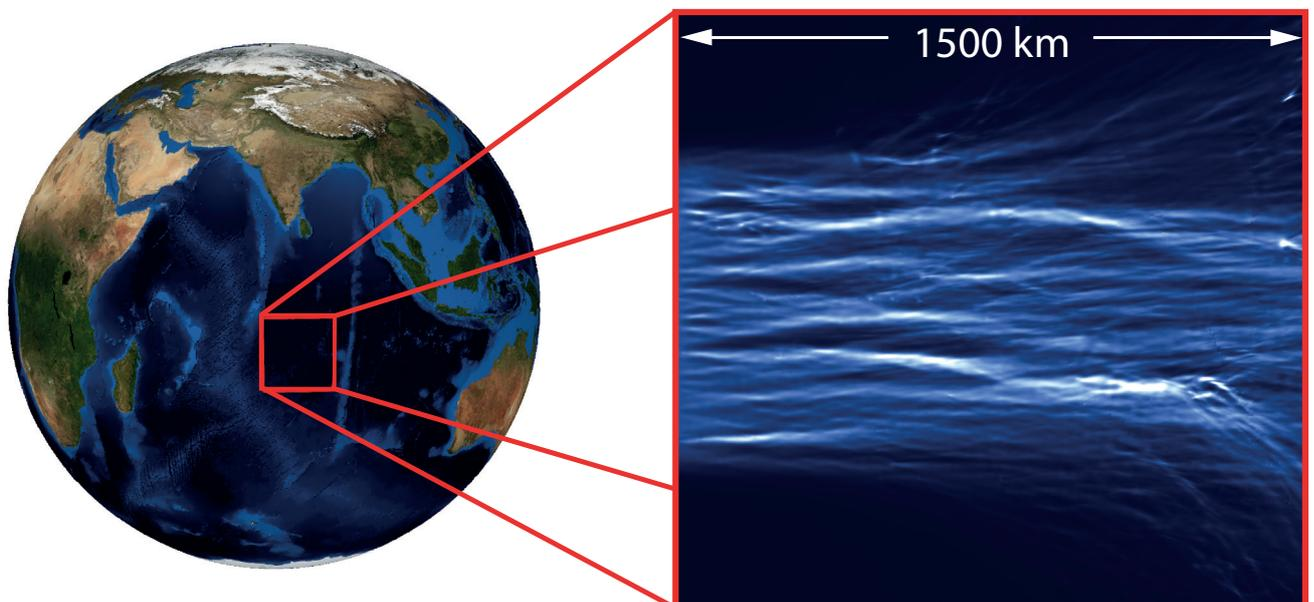
**Fig. 1:** The simulation of a tsunami wave in a region of the Indian Ocean where the ocean depth variations have a standard deviation of only less than 7% reveals the strong impact of branching on tsunami propagation [1].
