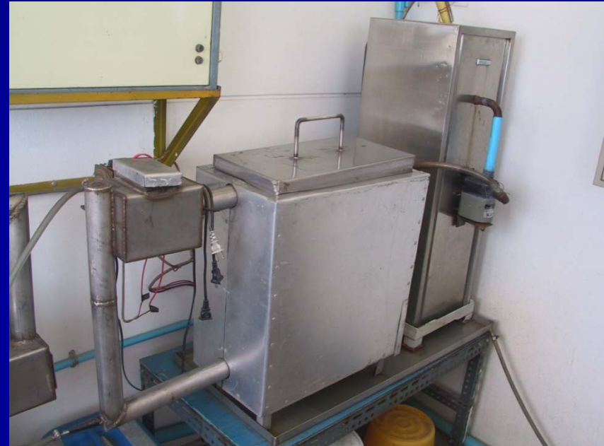
Steeping and germination unit
