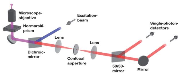
**Fig. 1** Principle of a confocal two focus experiment.
