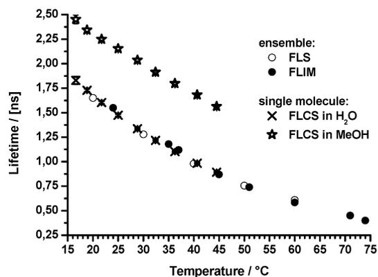
**Fig. 2** Fluorescence lifetime correlation spectroscopy (FLCS) measurements of Rhodamine B. Fluorescent lifetime measurements obtained from single molecule experiments in aqueous solutions (crosses) and in methanol (stars) compared with published fluorescence lifetime obtained from fluorescence lifetime spectroscopy (FLS)<sup>14</sup> and fluorescence lifetime imaging (FLIM),<sup>11,14</sup> as a function of temperature in aqueous solution (dots and circles).
