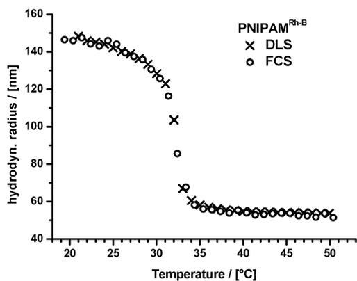
**Fig. 4** Labelled PNIPAM<sup>Rh-B</sup> microgels: DLS and 2fFCS measurements of thermosensitive microgel, with VPTT around 32 °C.
