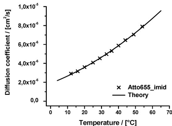
**Fig. 3** (*top*): 2fFCS measurement of Atto655\_imid, with a concentration of  $10^{-9}$  mol/l, autocorrelation functions, and 2f-cross-correlation function fitted with the 2fFCS-model, as described in eqn (1)–(4). (*bottom*): Temperature dependent measurement of Atto655\_imid fluorescence dye. Diffusion coefficient from 2fFCS is in perfect agreement with Stokes–Einstein equation.
