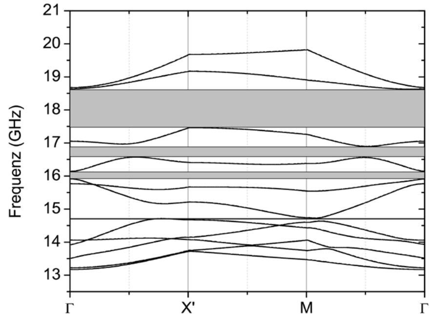
Band structure with  $a=3.5\mu\text{m}$  with  $kS=0.229$
