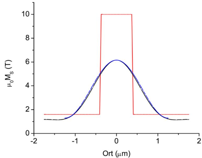
Profiles of simulated antidot for  $a=3.5\mu\text{m}$ ,  $R=0.4\mu\text{m}$  (11 lattice vectors,  $kS=0.233$ )
