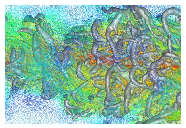
**Figure:** Thermal plume (tilted by 90°) with Lagrangian tracks of ~300,000 particles in a 0.6 m<sup>3</sup> volume, color coded with vertical velocity. Isosurfaces of Q-criterion show vortical structures.
