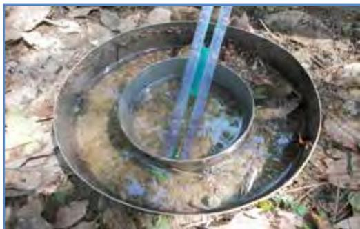
**Photo 36:** Measurement of soil water infiltration with a double-ring infiltrometer.
