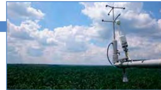
**Photo 11:** Eddy covariance instrumentation, including a sonic anemometer and infrared gas analyzer for H<sub>2</sub>O and CO<sub>2</sub> fluxes, installed at the top of the climate tower in PTPN VI.
