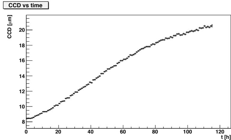
**Figure 6.5.:** Measurement of CCD of diamond sample 2 over time at a bias voltage of 700 V. Before the measurement the diamond was completely unpumped. An increase of CCD which is interpreted as pumping is visible. Only statistical errors are shown.
