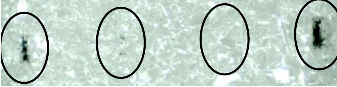
**Figure 7.5.:** Graphite spots for different powers of the laser beam. From left to right:  $(545 \pm 5) \mu\text{W}$ ,  $(482 \pm 5) \mu\text{W}$  (slightly visible),  $(367 \pm 4) \mu\text{W}$  (no transformation visible) and  $(584 \pm 6) \mu\text{W}$ . All spots were produced with an exposure time of 10 s, except the last spot which was exposed 20 s to the beam.
