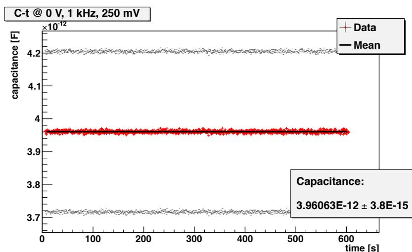
*Figure A.2.:* Measurement of capacitance at a constant bias voltage of 0 V and a frequency of 1 kHz. The error for each data point indicates the systematic uncertainty. The error on the capacitance is the statistical error.
