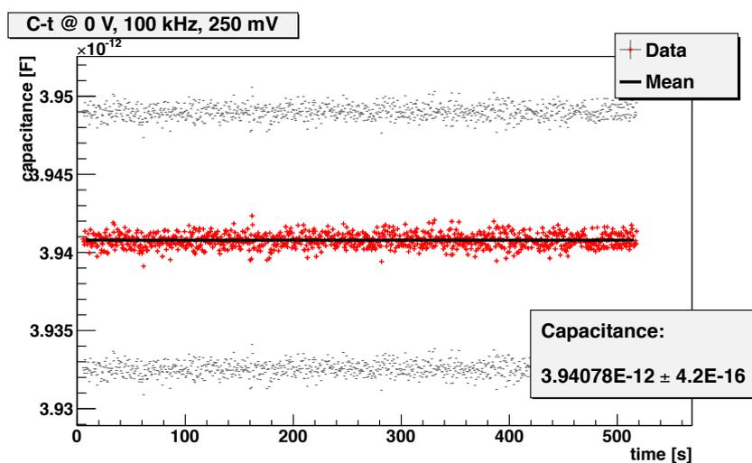
*Figure A.3.:* Measurement of capacitance at a constant bias voltage of 0 V and a frequency of 100 kHz. The error for each data point indicates the systematic uncertainty. The error on the capacitance is the statistical error.
