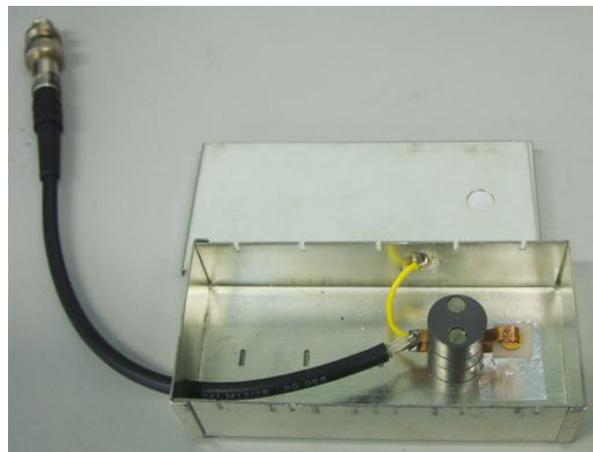
(b) Picture of the fixture for the CCD measurement. The samples are held by a Copper clamp. A hole in the clamp ensures that the material budget of the fixture is as low as possible.
