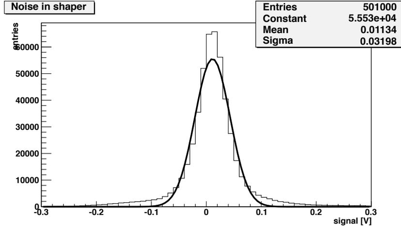
**Figure A.8.:** Noise after the shaper with diamond sample 1 connected and a bias voltage of 500 V. The shaper was set to a shaping time of 0.1  $\mu\text{s}$  and a nominal gain of 100. In this case two different sources of noise are visible. The dominating source has a much lower noise level than the suppressed source.
