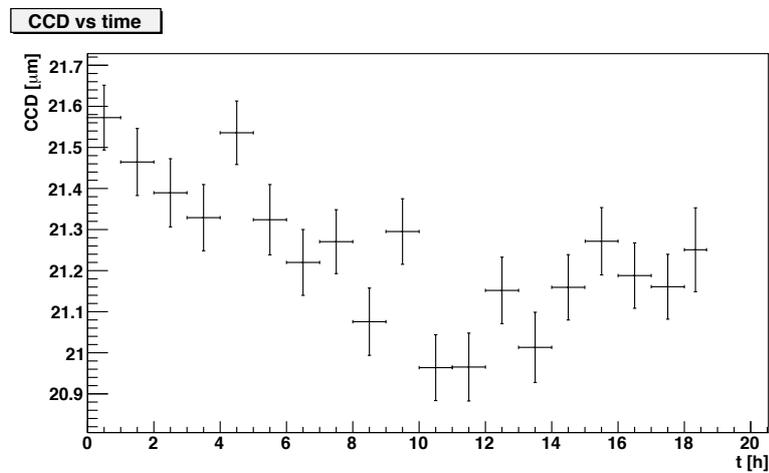
**Figure 6.8.:** Measurement of CCD of diamond sample 2 over time at a bias voltage of 1000 V. Before the measurement the diamond was pumped for more than 24 hours. A slight decrease of the CCD during the measurement is visible. Only statistical errors are shown.
