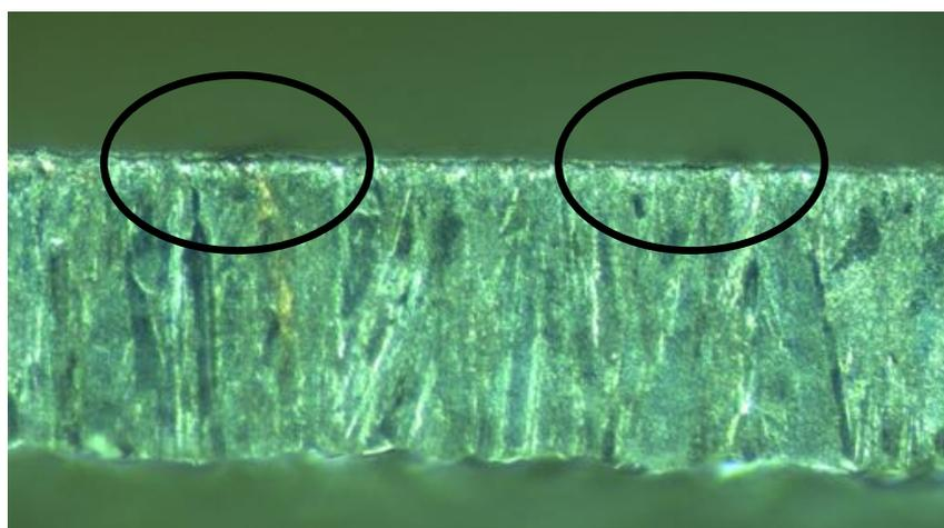
(b) Picture of the two spots from the side. The substrate side is on the top and the growth side at the bottom.
