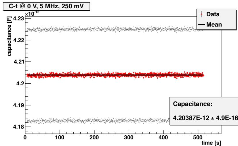
*Figure A.5.:* Measurement of capacitance at a constant bias voltage of 0 V and a frequency of 5 MHz. The error for each data point indicates the systematic uncertainty. The error on the capacitance is the statistical error.
