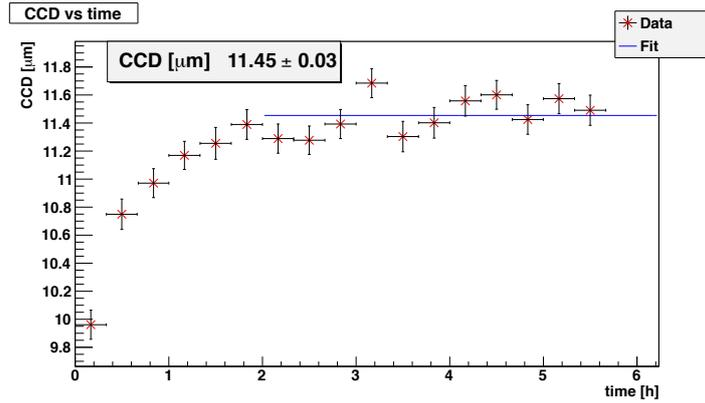
**Figure 6.10.:** Measurement of CCD of diamond sample 1 over time at a bias voltage of  $-200$  V. Prior to this measurement the diamond was fully pumped at a higher electric field. During the first two hours, an increase of CCD is visible. Only statistical errors are shown.
