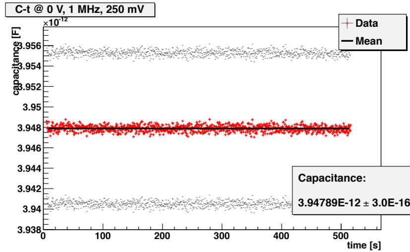
*Figure A.4.:* Measurement of capacitance at a constant bias voltage of 0 V and a frequency of 1 MHz. The error for each data point indicates the systematic uncertainty. The error on the capacitance is the statistical error.
