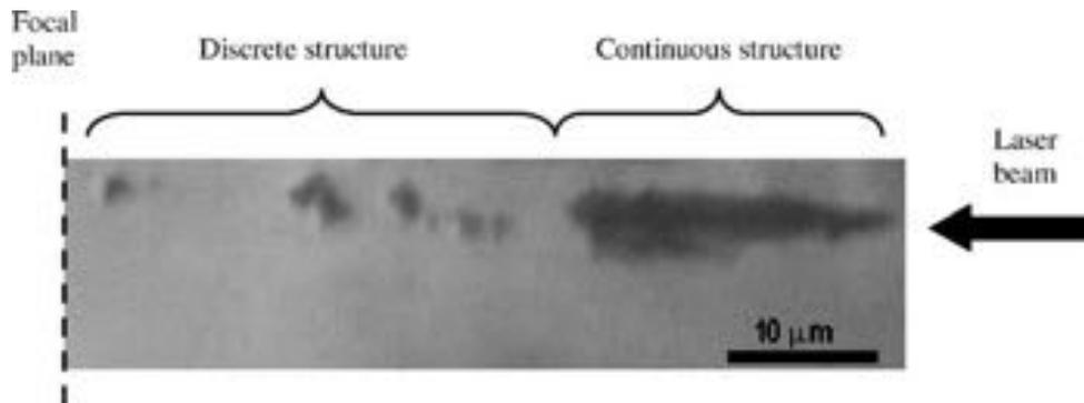
**Figure 4.3.:** Image of graphite impurities in diamond produced by multiple shots using a 120 fs laser. The separation into two types of structures is visible [32].
