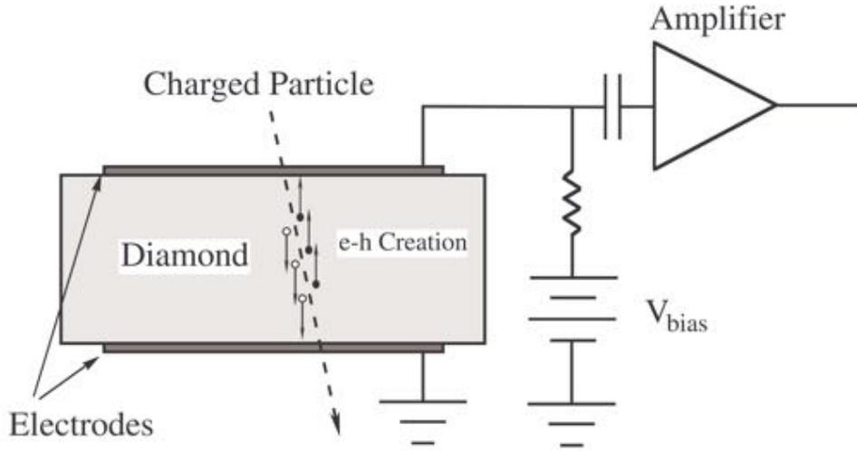
**Figure 2.3.:** Schematic illustration of a diamond detector with the first part of the electronic read-out. As the bias voltage is connected to the same electrode as the read-out, the capacitor decouples the amplifier from it [5].
