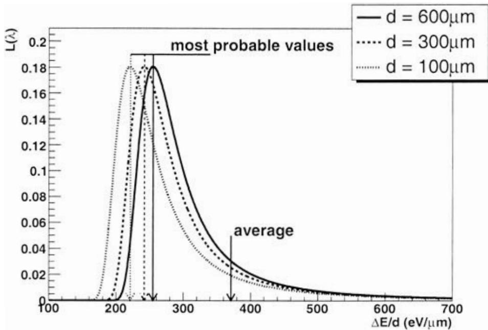
Figure 2.2.: Example for the Landau-distribution  $L(\lambda)$  of the energy loss of a m.i.p. in silicon with thickness  $d$ . The energy loss has been normalised to the sensor thickness  $d$ . The mean value and most probable values are indicated [4].
