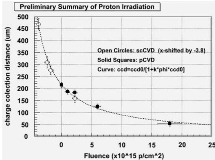
**Figure 4.1.:** Measured CCD before and after irradiation with 24 GeV protons for scCVD (open circles) and pCVD (solid squares) diamond. For both types the CCD at zero fluence is normalised to 220  $\mu\text{m}$ . The data for scCVD diamond is shifted to the left to match the damage curve of the pCVD diamond. This shows that both types have the same damage constant [16].
