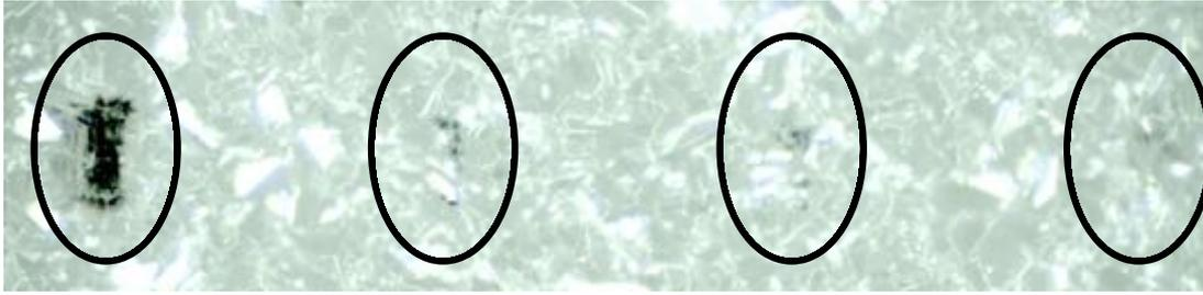
**Figure 7.6.:** Graphite spots for different times of exposure to the laser beam. From left to right:  $(584 \pm 6) \mu\text{W}$  for 3 s,  $(482 \pm 5) \mu\text{W}$  for 60 s, 40 s and 20 s (no transformation visible).
