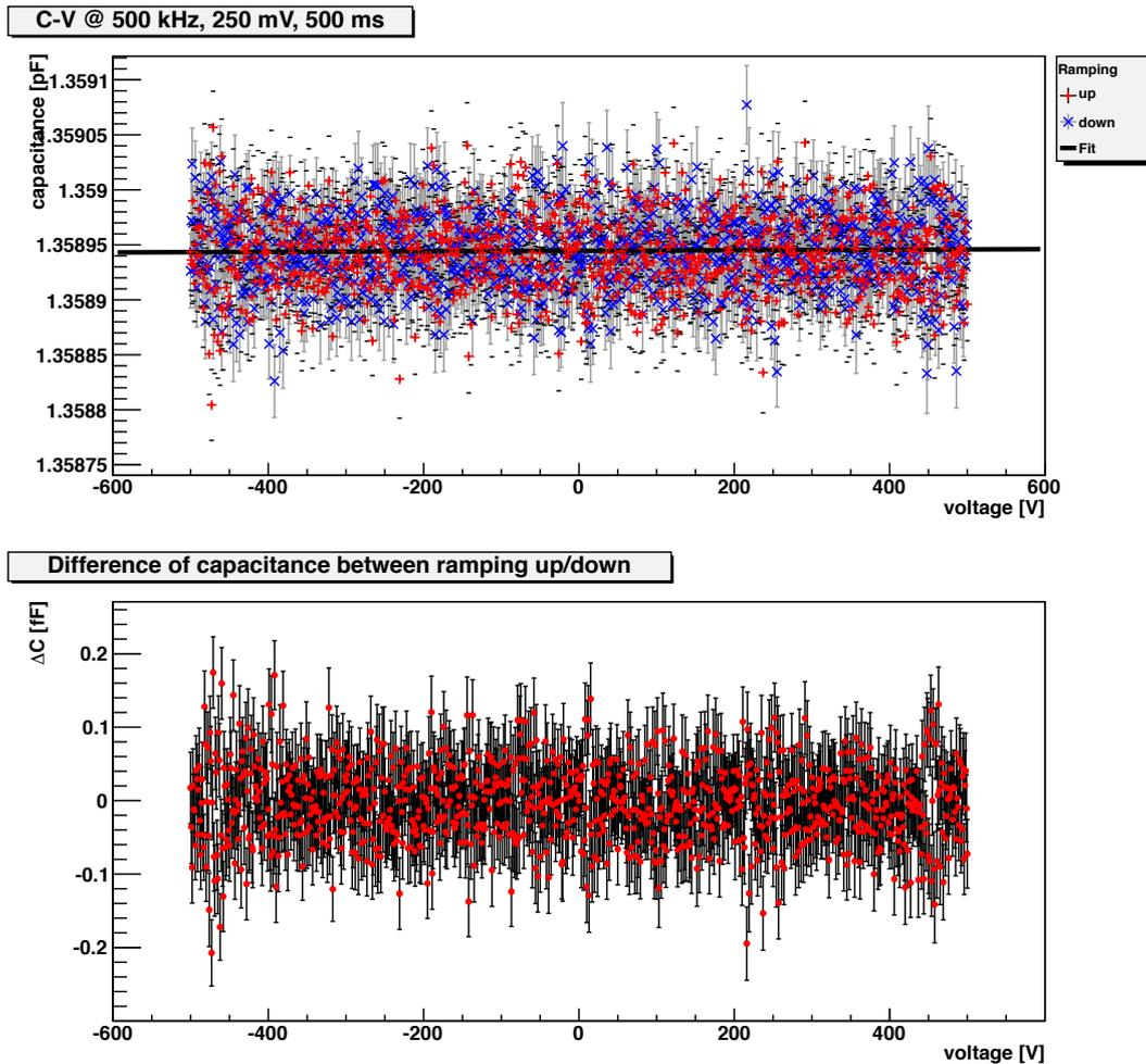
**Figure 5.8.:** Voltage sweep from  $-500$  V to  $500$  V for the non irradiated diamond sample 3. The sweep was repeated 235 times. The upper plot shows the measured capacitance for each step with a step size of  $1$  V. The lower indicates the difference for the values between ramping up and down. Only statistical errors are shown.
