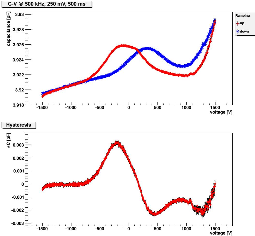
**Figure 5.10.:** Measurement with the same parameters as in Figure 5.9 but with flipped diamond. This means that the high voltage is applied on the other electrode. The sweep was repeated 139 times. Only statistical errors are shown.
