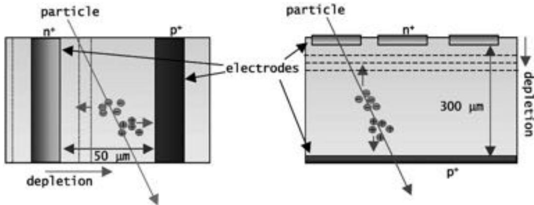
**Figure 4.2.:** Sensor with 3D (left) and planar (right) electrodes. In both cases the same amount of charge is deposited by the incoming particle as it has to pass the full sensor thickness. But for the 3D electrodes these charges are generated much closer to the electrodes. As the spacing between them is lower, for semiconductors the depletion voltage decreases [19].
