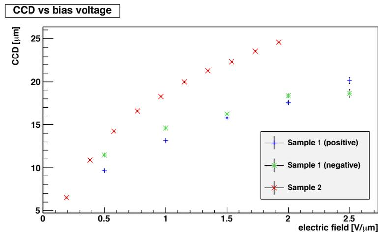
**Figure 6.9.:** CCD for completely pumped samples with respect to the electric field. For diamond sample 1, a positive and negative bias voltage is applied to collect electrons and holes, respectively. Only statistical errors are shown.
