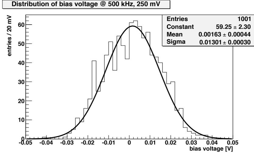
**Figure 5.6.:** Distribution of the measured bias voltage during one capacitance measurement at 0 V. The uncertainty of the voltage supply exceeds the uncertainty induced by a voltage sweep from 0 V to 1 mV.
