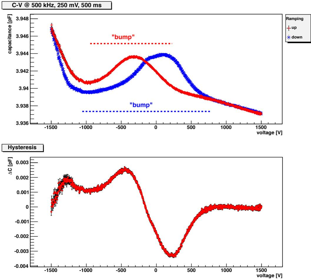
**Figure 5.9.:** Voltage sweep from  $-1500$  V to  $1500$  V for the highly irradiated diamond sample 1. The sweep was repeated 122 times. The upper plot shows the measured capacitance for each step with a step size of  $3$  V. The lower indicates the difference for the values between ramping up and down. Only statistical errors are shown.
