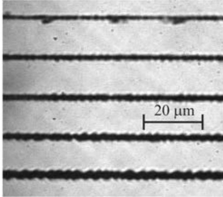
**Figure 4.4.:** Graphite tubes in diamond produced with an 800 nm laser which is pulsed with 140 fs at a repetition rate of 1 kHz. From top to bottom the speed of the moving sample was  $1 \frac{\mu\text{m}}{\text{s}}$ ,  $3 \frac{\mu\text{m}}{\text{s}}$ ,  $5 \frac{\mu\text{m}}{\text{s}}$ ,  $10 \frac{\mu\text{m}}{\text{s}}$  and  $30 \frac{\mu\text{m}}{\text{s}}$  [33].
