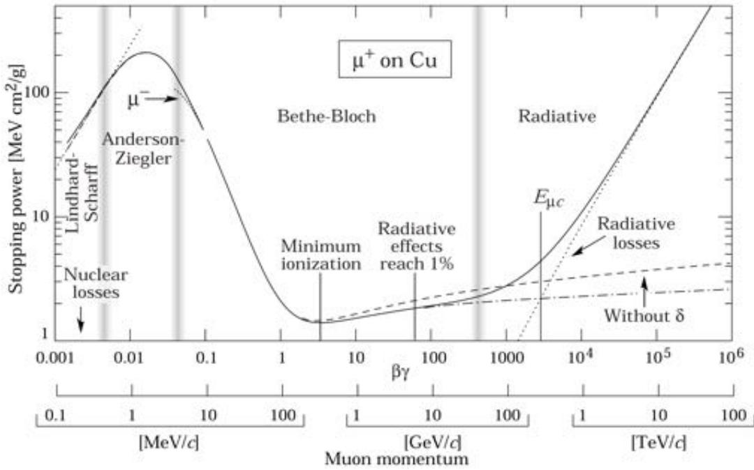
Figure 2.1.: Energy loss of muons in Copper [3].
