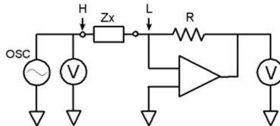
**Figure 5.4.:** Simplified sketch of the measurement of impedance  $Z_x$  using the auto balancing bridge method. A virtual ground is generated at point  $L$ , thus the same current flows through the unknown impedance  $Z_x$  and the known resistor  $R$ . The impedance is calculated from the potential over the resistor  $R$  and over  $Z_x$  [35].
