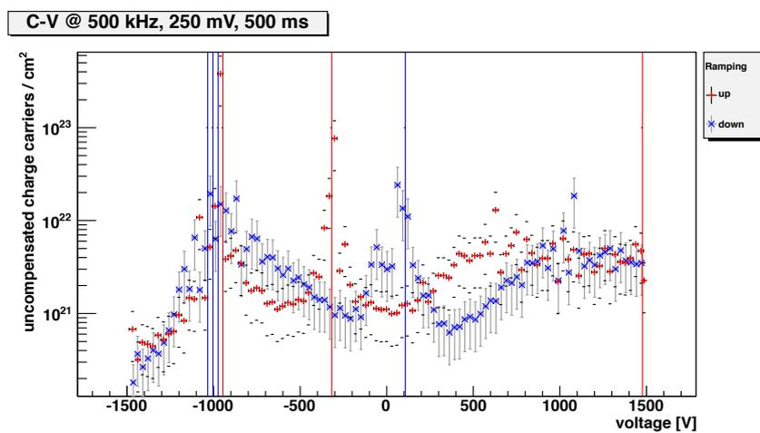
**Figure A.6.:** Uncompensated charges as a function of the bias voltage. A change of the sign of the uncompensated charge according to the theoretical model is indicated by vertical lines in the colour of the direction of the voltage sweep.
