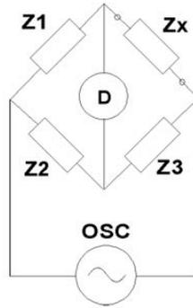
**Figure 5.3.:** Measurement of impedance  $Z_x$  using the bridge method. The three known impedances  $Z_i$  are adjusted, such that no current flows in the detector  $D$  [35].
