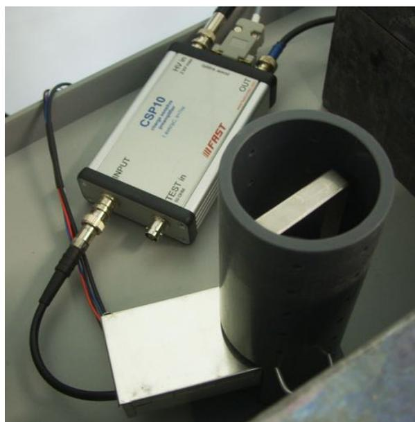
(a) Picture of the plastic tube with source and metal box inserted and the preamplifier. Not visible are the collimator and the scintillator under the box.
