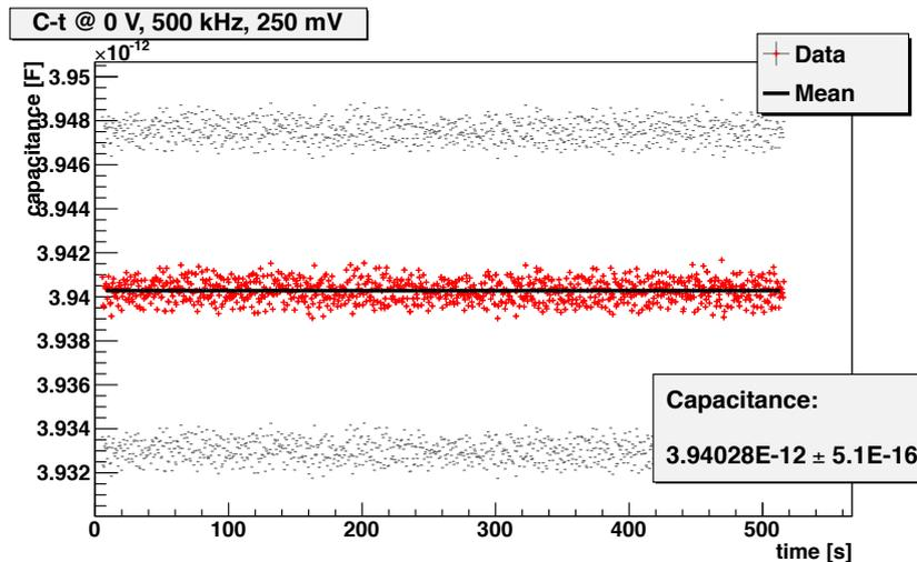
**Figure 5.7.:** Measurement of capacitance at a constant bias voltage of 0 V and a frequency of 500 kHz. The error for each data point indicate the systematic uncertainty. The error on the capacitance is the statistical error.
