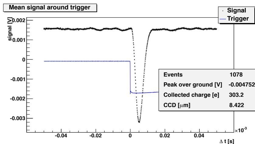
**Figure 6.6.:** Mean values of all 1078 events from the first hour of the measurement in Figure 6.5. Note that each event already contains the mean values of 128 single events. For each point of the curve, the corresponding data of the 1078 events are histogrammed and fitted with a Gaussian distribution. The mean signal of the trigger is printed in blue.
