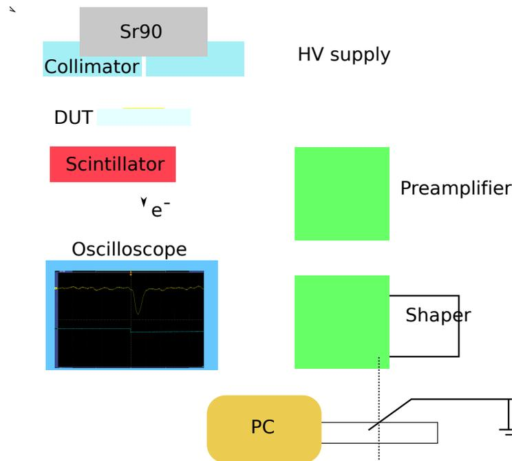
**Figure 6.3.:** Illustration of the read-out chain. The signal from the diamond is processed in a charge sensitive preamplifier and a shaper. As an external trigger, a scintillator is used. Both signals are recorded by an oscilloscope and transferred to a computer.
