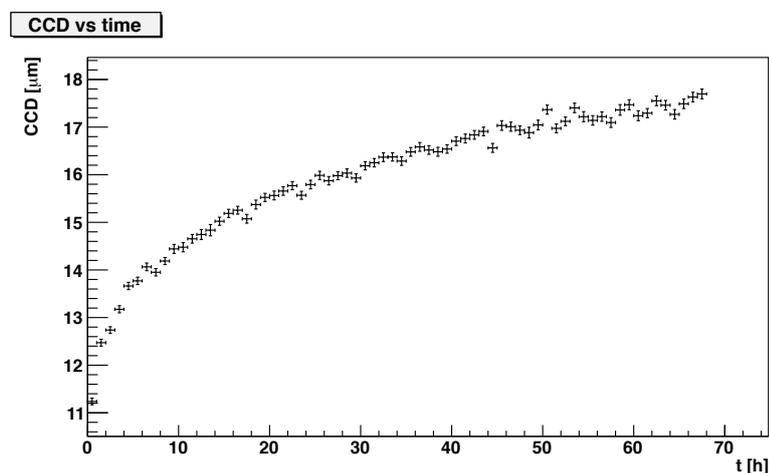
**Figure 6.7.:** Measurement of CCD of diamond sample 1 over time at a bias voltage of 700 V. Before the measurement the diamond was completely unpumped. An increase of CCD and thus a pumping effect is visible. Only statistical errors are shown.
