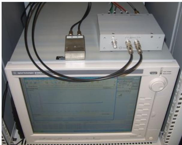
**Figure 5.1.:** Photograph of the B1505A. On top of it lies the metal box including the fixture for the diamonds and a bias tee to connect it with the B1505A.
