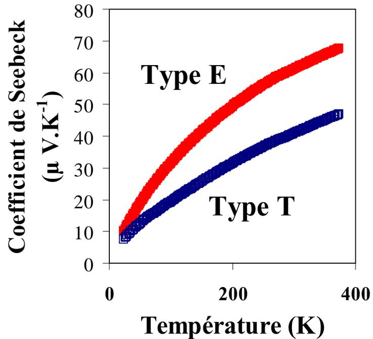
Thermopile – non-linear response in function of the temperature
