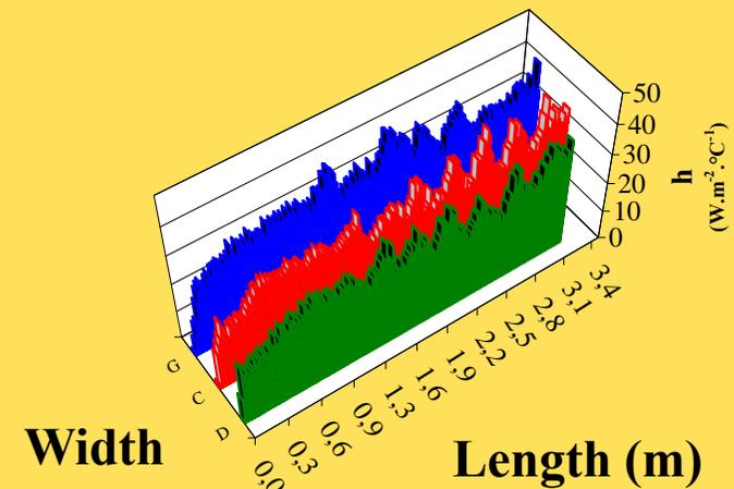
**Coefficients air side** – low efficiency zones as a result of the position of ventilators (high standard deviation increases ft in 5-15%)
