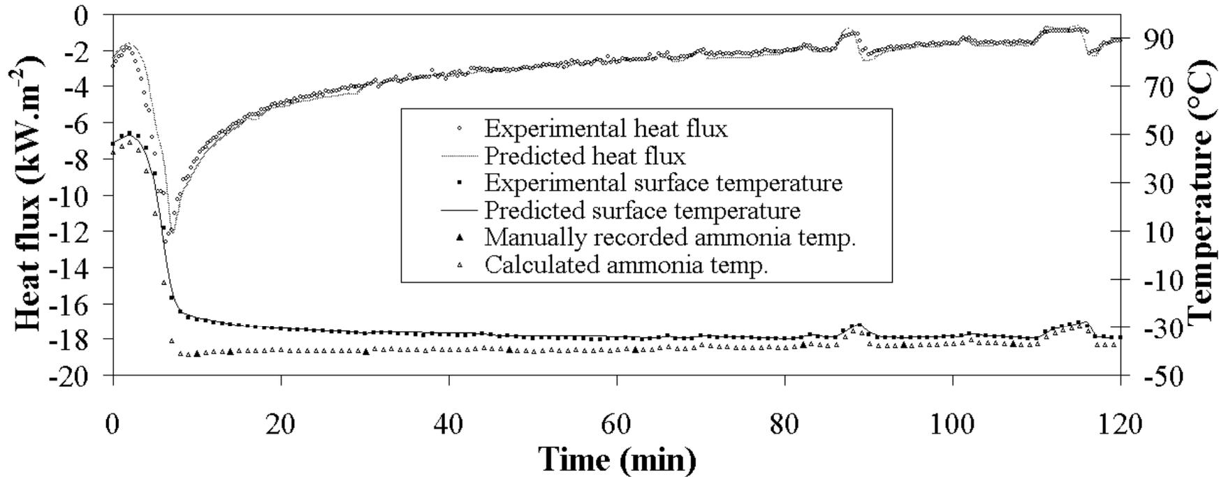
$h = 560 \text{ W/m}^2\text{°C}$  – compatible with contact freezing
