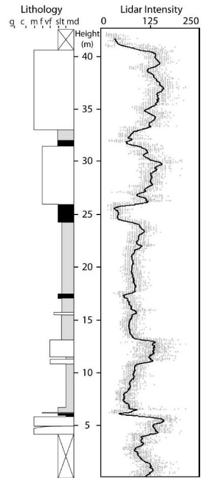
FIG. 7.—Lithology log (from measured section) and lidar intensity log of the Prince Creek Formation.
