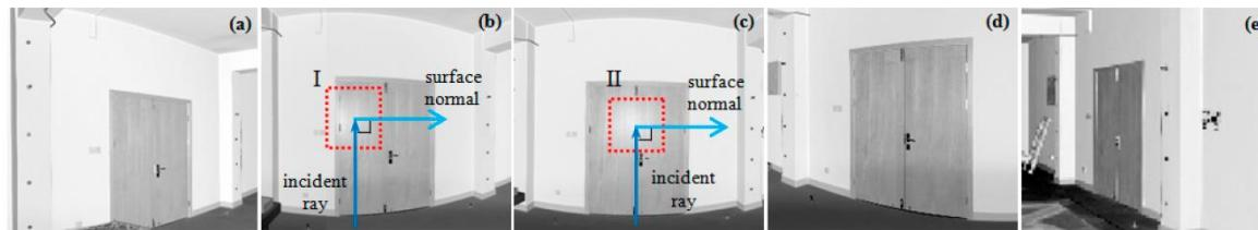
**Figure 3.** Original intensity images created by Faro SCENE. (a) Scan 1. (b) Scan 2. (c) Scan 3. (d) Scan 4. (e) Scan 5. Highlights exist in Scans 2 and 3 because the surface of the door is smooth. Scans 1, 4, and 5 do not have highlight regions as the surface of the wall is relatively rough.
