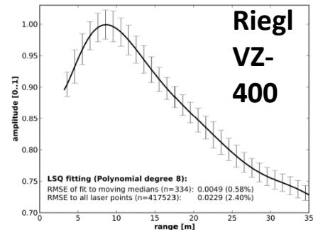
Figure 6. Variation of raw intensity data with distance for all of the three reference targets with the reflectance of 15%, 30% and 60% at the incident angle of 0°.
