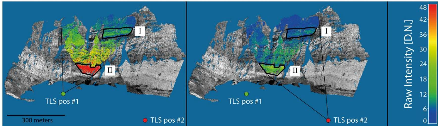
**Fig. 9.** Illustration of the same scanned surface with raw intensities of the Dents-du-Midi acquired from two different points of view (TLS position #1 and #2) overlaying corrected intensity scans. The comparison of the same areas between scan positions #1 and #2 shows different raw intensity values which are related to range, incidence angle and surface geometry differences.
