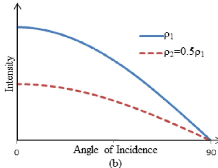
**Figure 6.** (a) Theoretical relationship of intensity measurements vs. range shown for two materials with different reflectance ( $\rho$ ); and (b) theoretical relationship of intensity measurements vs. angle of incidence shown for two materials with different reflectance ( $\rho$ ).
