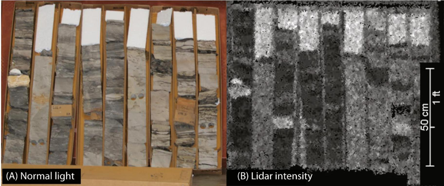
FIG. 3.—Boxes of core were used in experiment 1. A) Shale in the core corresponds to low intensities B) The intensity grayscale is 0 (black) to 255 (white).
