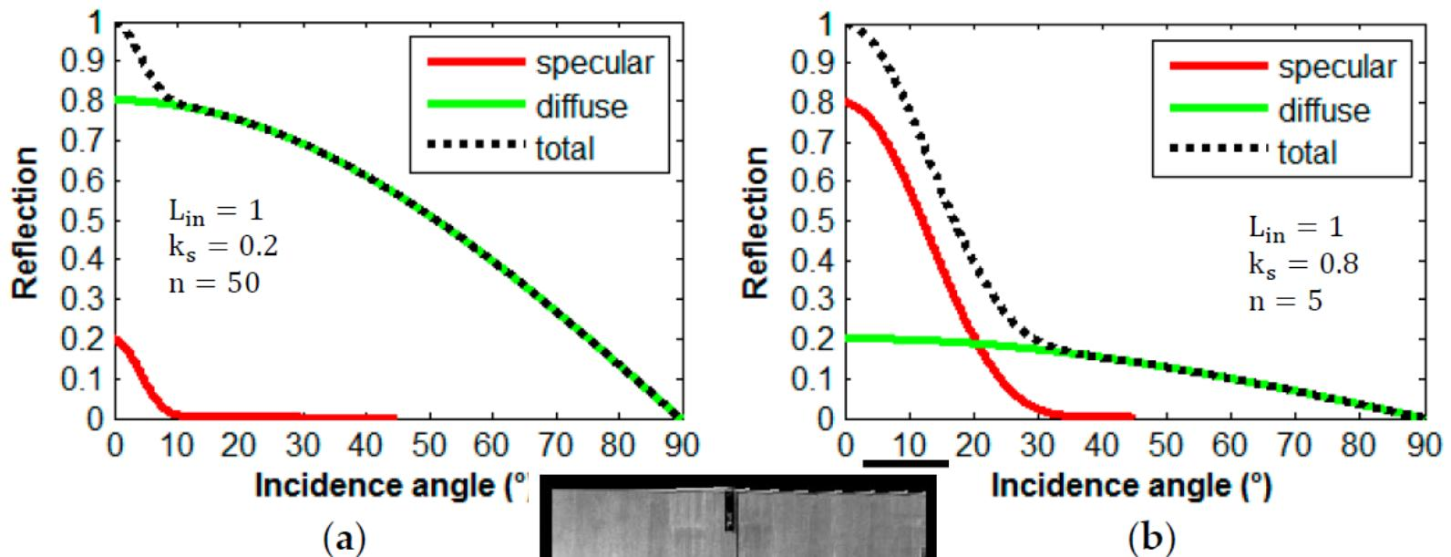
Figure 2. Phong model with different angles smaller than  $45^\circ$  and must be considered (rough surfaces).
