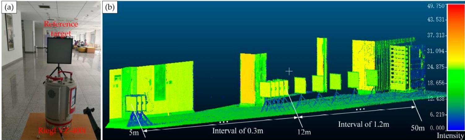
**Figure 4.** Experimental setup and scene of the distance experiment. (a) experimental setup including Riegl VZ-400i and three reference targets with reflectance of 15%, 30% and 60%, respectively; (b) scene of the distance experiment with distance from 5 m to 50 m, and a step interval of 0.3 m from 5 m to 12 m, and 1.2 m from 12 m to 50 m, respectively.
