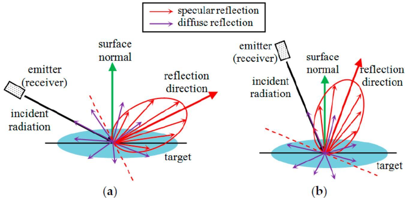
**Figure 1.** (a) At incidence angles larger than  $45^\circ$ , only diffuse reflections reach the receiver. (b) At incidence angles smaller than  $45^\circ$ , both diffuse and specular reflections can be received. The red dotted lines are perpendicular to the reflection directions.
