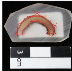
**Figure 1. Sampling for the Biodur-embedded bones.** The excess epoxy resin and every outer surface of the embedded bones was removed (red dotted lines).
