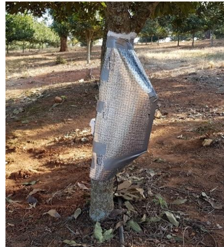
Protected sap-flow sensor on a macadamia tree.
