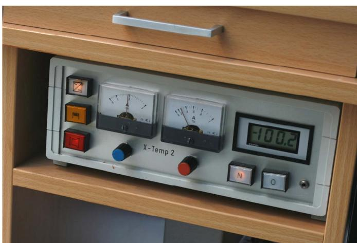
crystal cooling by a  $N_2$  inert gas stream generated by *X-Temp 2*
