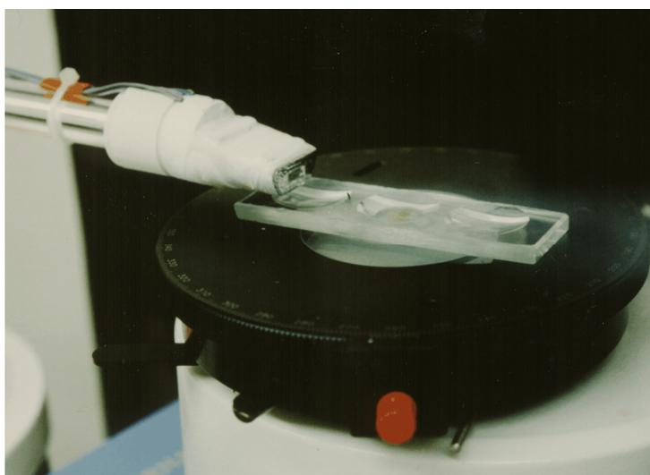
Single crystals immersed in an inert oil *X-Temp 2* cooled on the microscope slide
