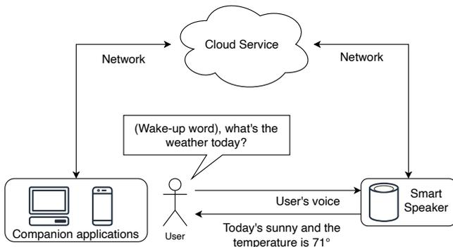
Fig. 2. Smart speaker architecture based on [6]
