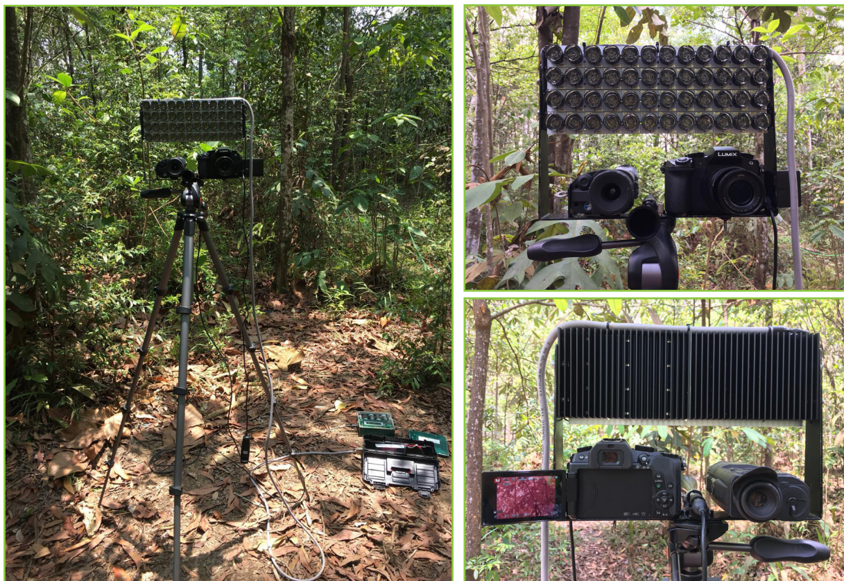
Figure 1. Point count methods using a thermal imagery, camera, LED lamps and song meter
