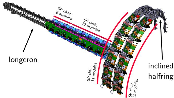
**Figure 3.11.:** CAD view of the ITk OB demonstrator with one longeron and two half rings. The longeron will have one full SP-chain with 12 modules and a smaller SP-chain, which can be filled with up to 6 modules. The inclined half rings will have one SP-chain each, with one SP-chain being full (11 modules).
