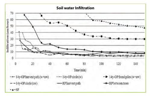
**Figure 46:** Infiltration in different forest transformation systems: OP – oil palm, RP – rubber monoculture, SF – secondary forest, w – weeded, uw – unweeded, 14y – 14-year-old.
