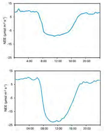
**Figure 5:** Mean diurnal cycles of  $CO_2$  net ecosystem exchange (NEE) in the (a) 2-yr old non-productive and (b) 12-yr old mature plantations. Negative values indicate  $CO_2$  uptake, positive values  $CO_2$ , release.
