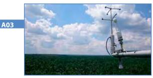
**Photo 11:** Eddy covariance instrumentation, including a sonic anemometer and infrared gas analyzer for  $H_2O$  and  $CO_2$  fluxes, installed at the top of the climate tower in PTPN VI.
