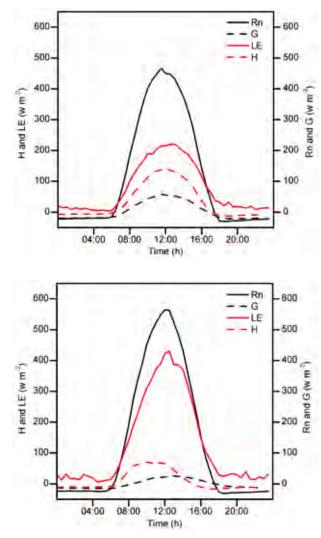
**Figure 4:** Mean diurnal cycles of sensible heat flux (H), latent heat flux (LE), net radiation (Rnet) and soil heat fluxes (G) in the (a) 2-yr old non-productive and (b) 12-yr old mature plantations.
