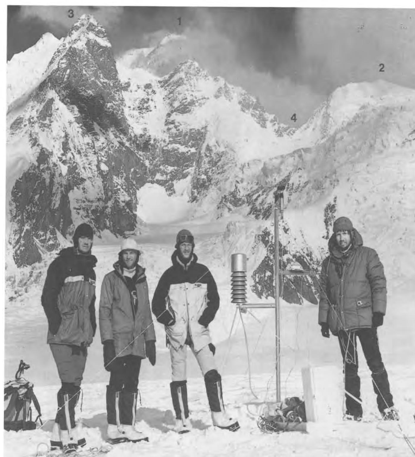
◀ Fig 33 The fourth, and highest, of the expedition weather stations on the orographic left-hand tributary branch in the feeding area at 5330 m asl (cf. Fig 1a □, left), weighs 75 kg and was taken up on a sledge pulled by the German and Chinese scientists. It operated for 17 days, from 21.9 to 7.10.1986. Every 20 minutes the 12 different measurement data were averaged and stored together with the extreme values. Their batteries were charged by S-facing solar collectors and were thus maintained in working condition. No. 1 = Skyang Kangri 7544 m; No. 2 = 6869 m peak; No. 3 = c. 6400-6600 m high peaks in the ridge between Skyang Kangri glacier and K2 glacier as they are running between Skyang Kangri and the 6640 m peak; No. 4 = 6526 m saddle towards the Godwin-Austen glacier (Baltoro glacier system); beneath this high relief there is the firm cauldron of the orographic right-hand (eastern) tributary branch of the K2 glacier. Viewpoint: 35°54'45"N/76°28'30"E. Photo: M. Kuhle 21.9.86.
