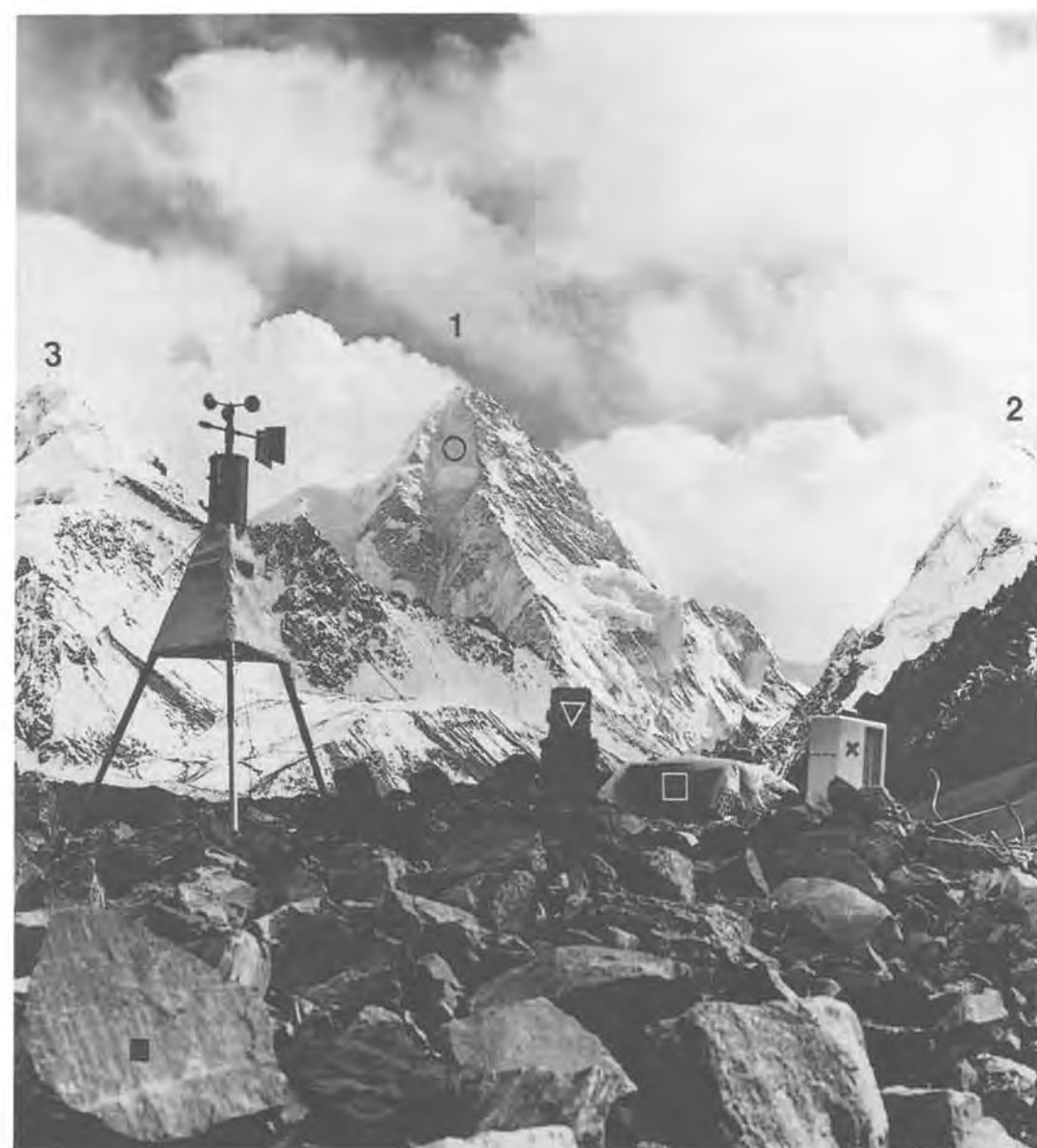
Fig 28 ▲ From 7.9.–11.10. 1986 the third weather station (from the base) of the 1986 expedition operated on the surface moraine drift (■) in the centre of the 2 km-wide K2 glacier at 4620 m asl (cf. Fig 30 x left). Next to the 12 channels station of the “Lambrecht” type, complete with wind metre and shaded thermohydrograph (on the left side), an independent mechanical actinography (▽) was installed in order to carry out checks on the measurement of global radiation, together with a termograph (x) for the recording of the temperature of the surface moraine at the different drift levels. Data storage was effected with a data logger (□). No. 1 = K2; No. 3 = 6640 m peak; No. 2 = c. 6800 m peak. Viewpoint: 36°00'30"N/76°33'15"E. Photo: M. Kuhle 11.10.86.
