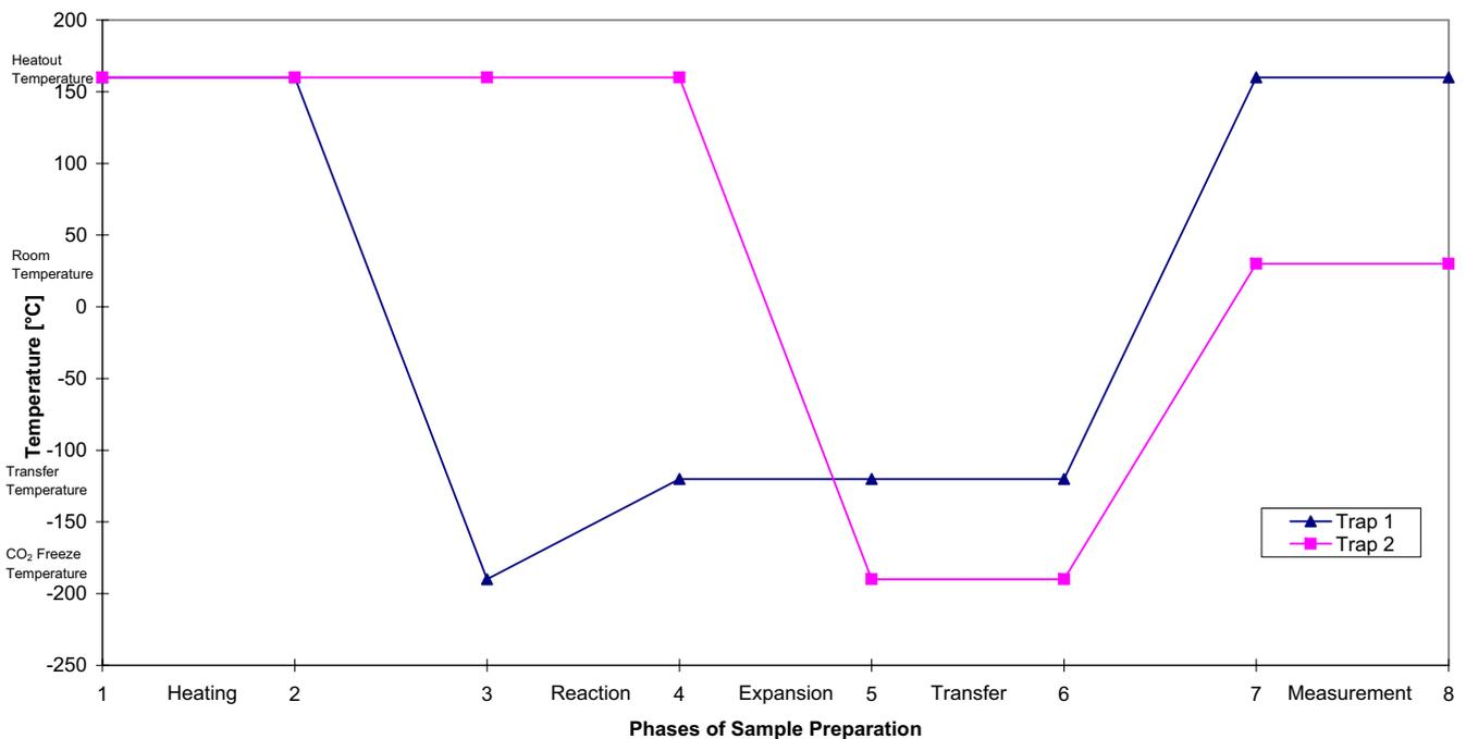
Figure 5-7. Trap Temperatures during Sample Preparation
