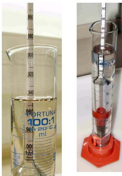
**Figure 4-27.** Checking Specific Gravity of Phosphoric Acid
