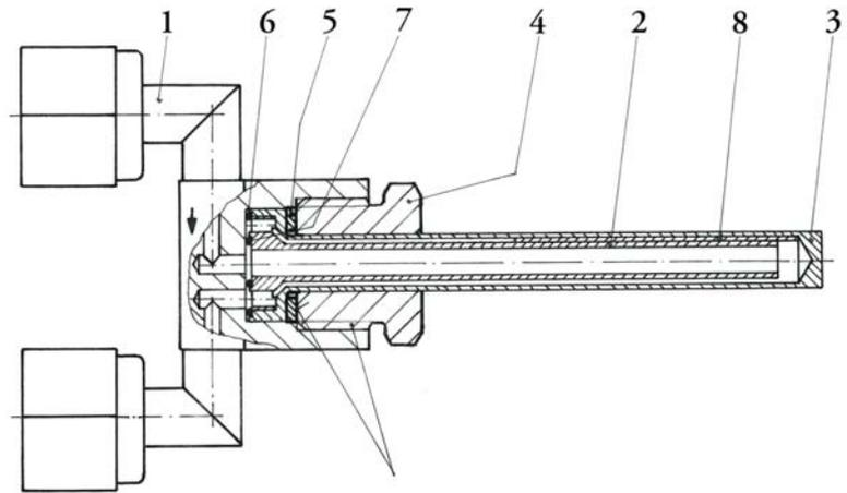
**Figure 6-19.** Trapping Volume (Part No. 100 7740)
