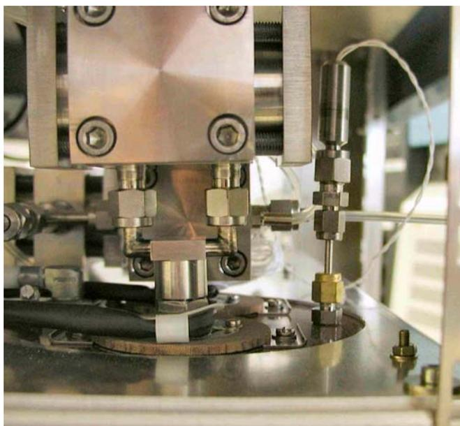
**Figure 2-51.** Position of Refill Sensor
