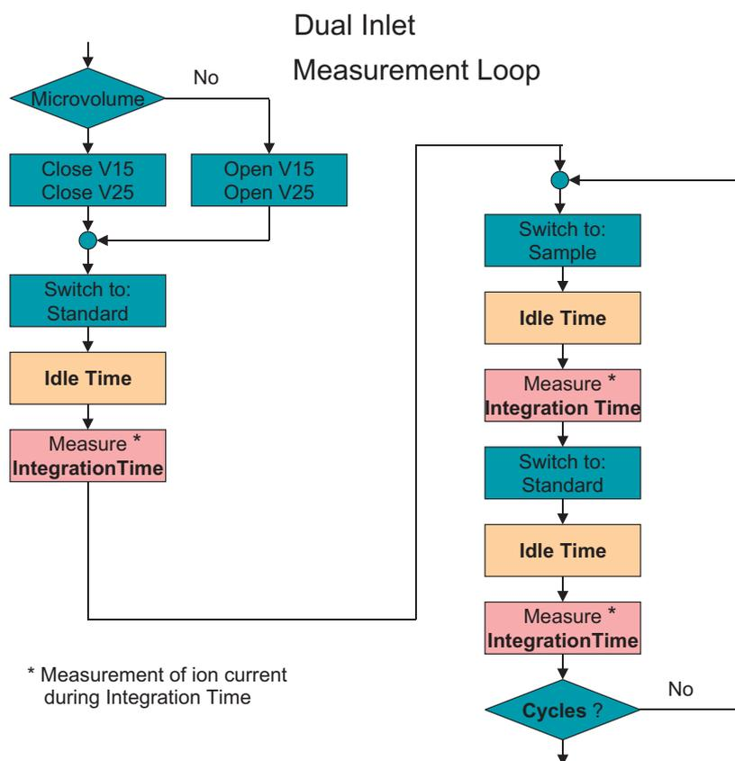
**Figure 3-13.** Dual Inlet Measurement Loop
