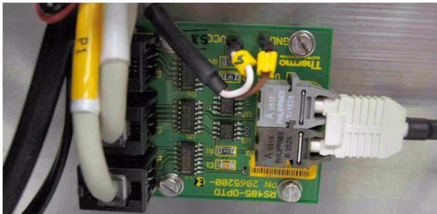
**Figure 2-11.** Fiberline to Serial Bus Interface
