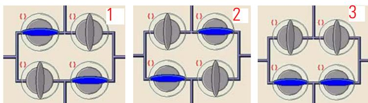
**Figure 3-12.** Switching Positions of Changeover Valve
