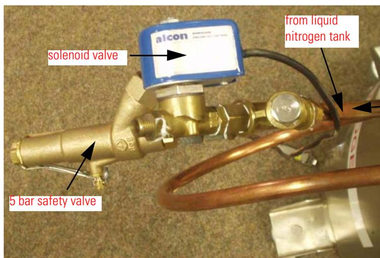
**Figure 2-48.** Valves and Distributor for Liquid Nitrogen (Top View)
