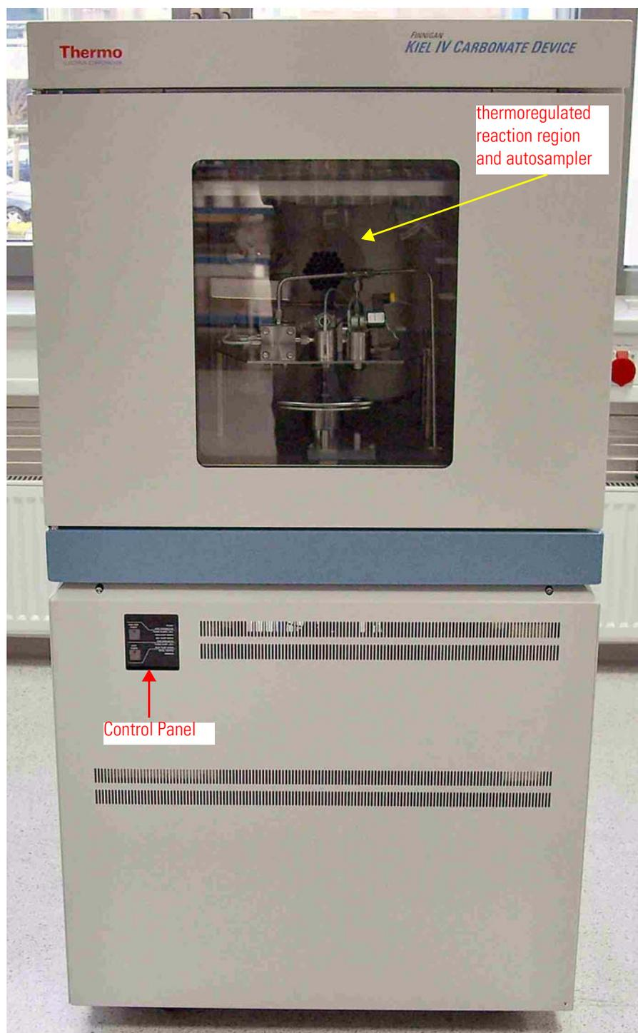
**Figure 5-1.** Finnigan Kiel IV Carbonate Device - Front View
