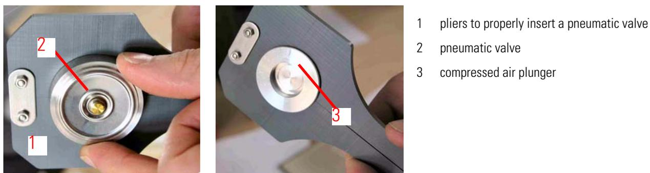
Figure 2-22. Pliers to Insert a Pneumatic Valve
