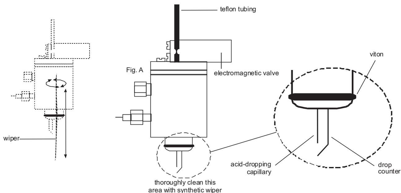
**Figure 4-21.** Cleaning Acid Valve
