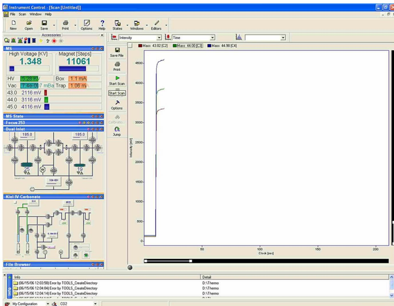
Figure 4-4. Instrument Control as Aid when Leak Checking
