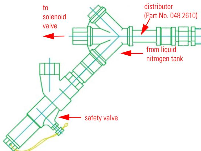
**Figure 2-50.** Valves and Distributor for Liquid Nitrogen
