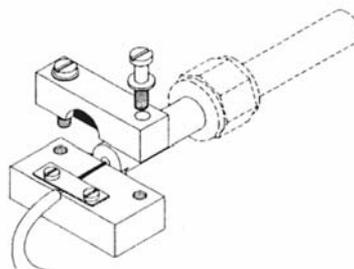
**Figure 4-11.** Crimping Device at the End of a Capillary
