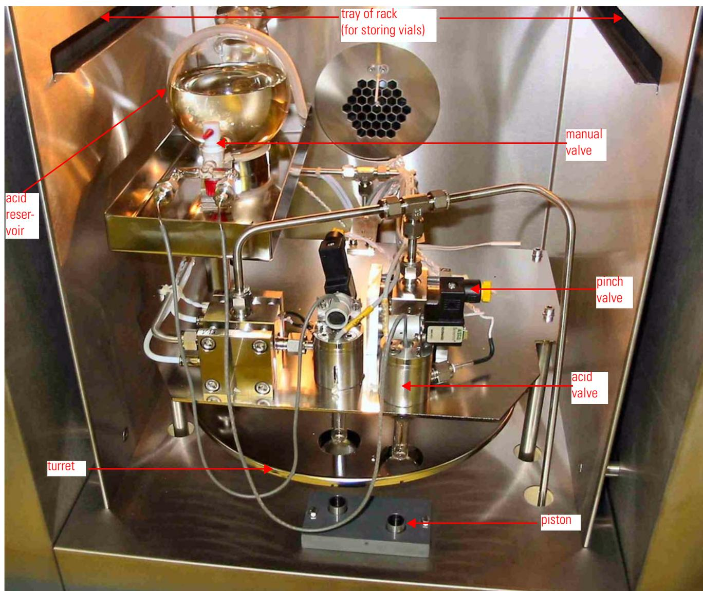
**Figure 2-2.** Heating Cabinet - Front View
