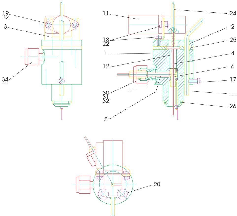
Figure 6-18. Acid Valve (Part No. 106 9450)
