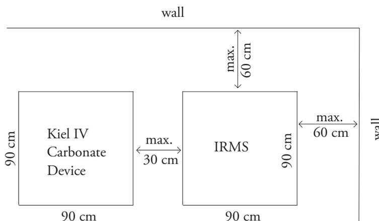
**Figure 1-1.** Kiel IV Carbonate Device - Site Requirements
