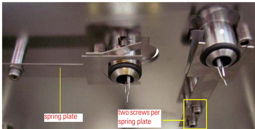
**Figure 4-18.** Mounted Spring Plate - Bottom View
