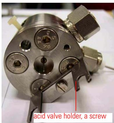
Figure 4-15. Acid Valve - I\*
