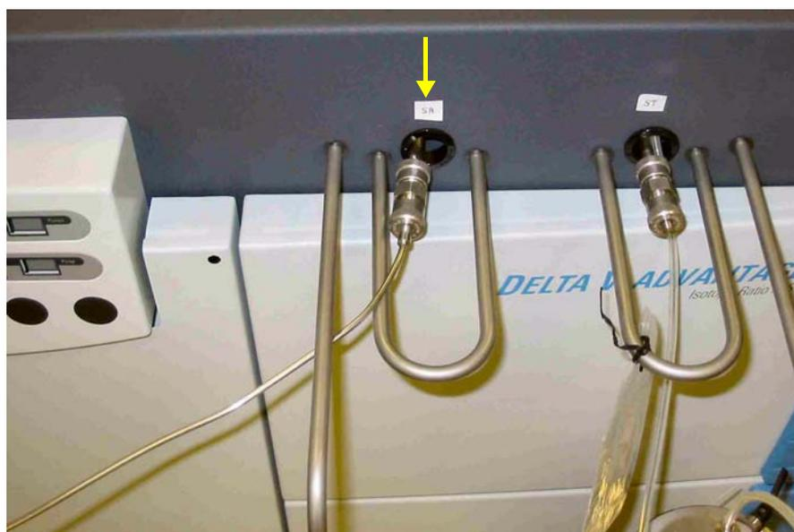
**Figure 4-8.** Connecting Transfer Tube to IRMS
