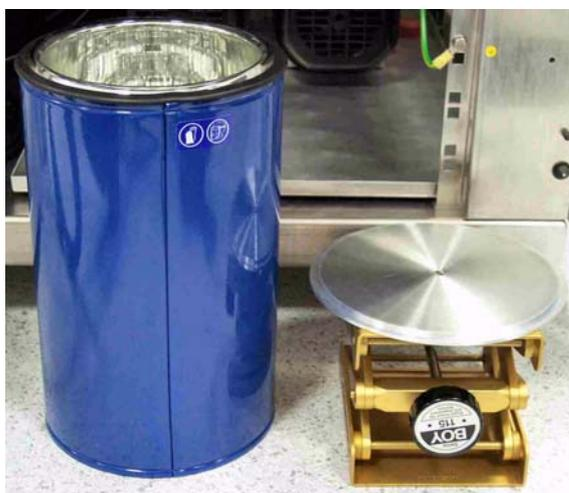
A dewar serves as reservoir for liquid nitrogen. It is adjusted beneath the trap assembly using a "lab boy".
