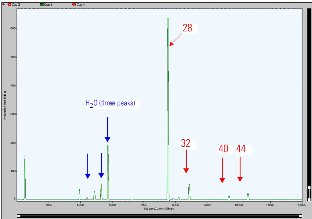
Figure 4-1. Mass Spectrum of Background Gas Composition \*
