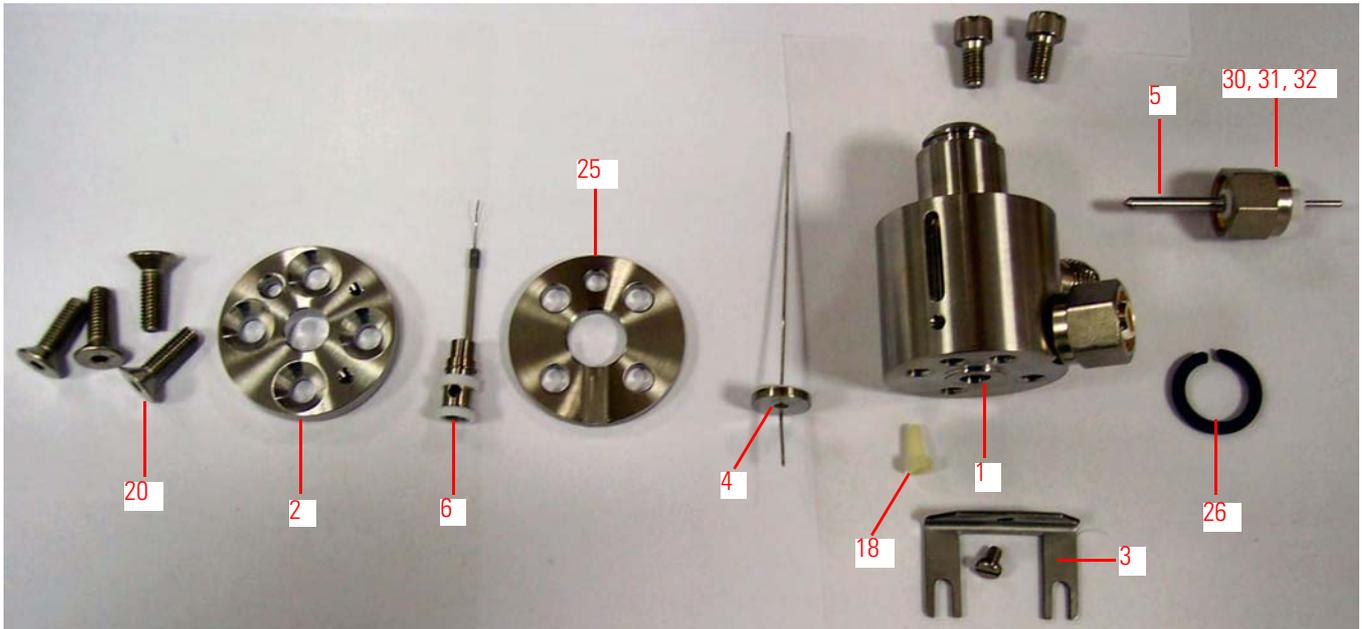
Figure 6-17. Parts of Acid Valve
