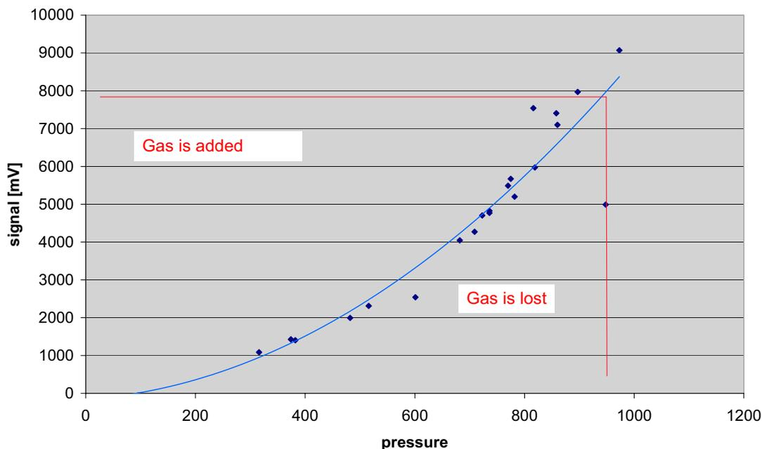
Figure 5-10. Signal vs. Pressure
