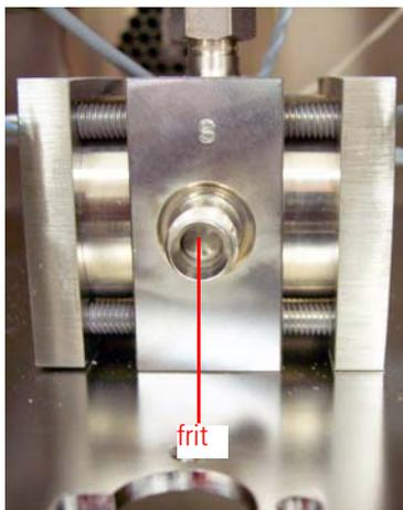
**Figure 4-20.** Valve Flange with Frit
