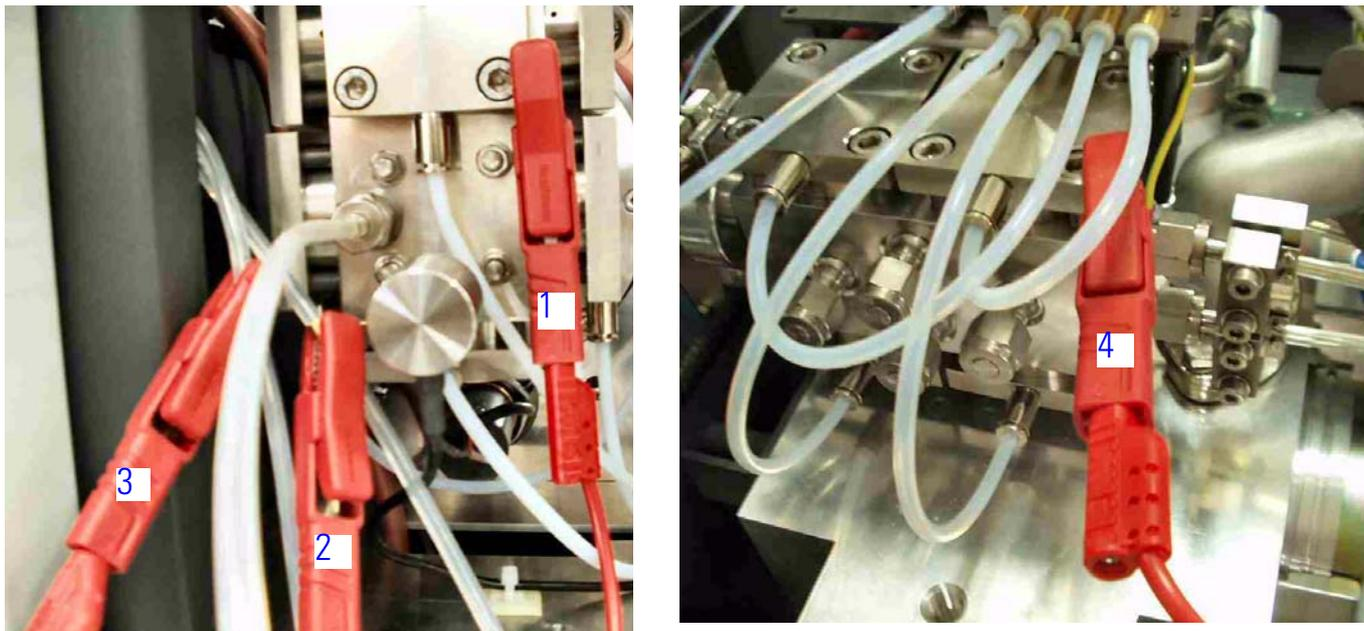
**Figure 2-17.** Fixing Alligator Crimps to Capillaries
