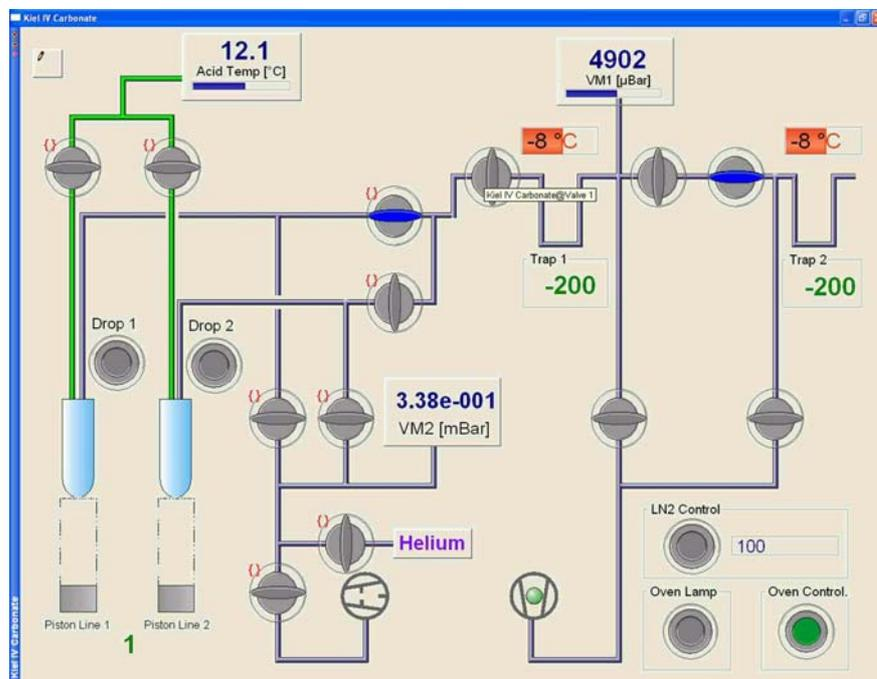
Figure 6-34. Checking V1 - Step 1
