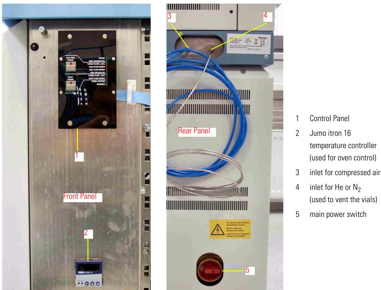
Figure 2-7. Parts of Front Panel and Rear Panel
