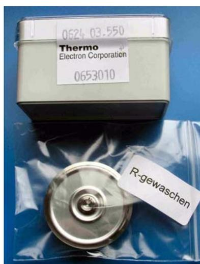
**Figure 6-9.** Complete Membrane (Part No. 065 3010)
