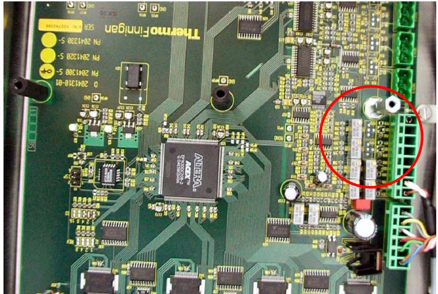
Figure 6-39. Adjusting Sensitivity of Drop Counters
