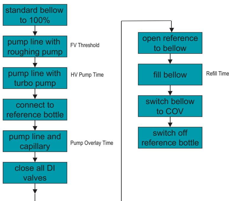
**Figure 5-15.** Reference Refill Process\*
