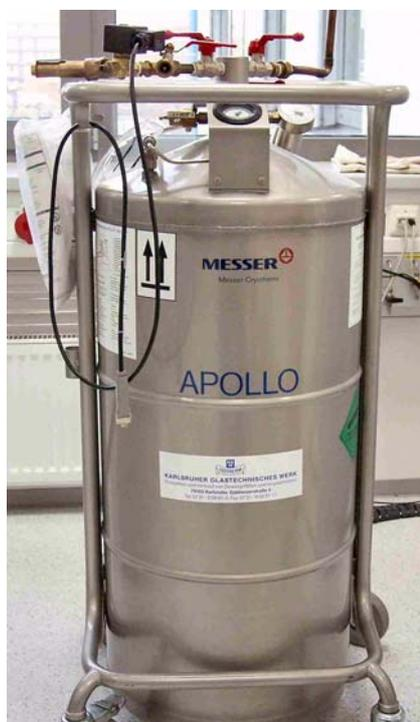
**Figure 2-47.** Example of a Liquid Nitrogen Refill Device
