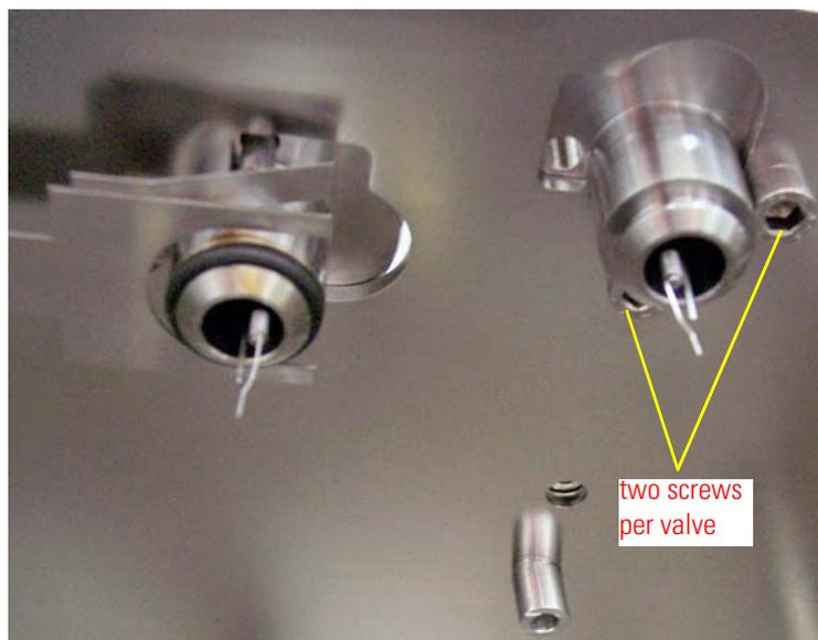
**Figure 4-19.** Mounted Valve - Bottom View
