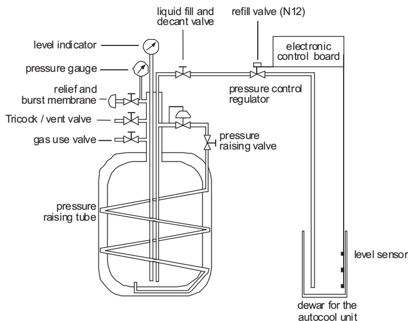
**Figure 2-45.** Schematic of a Standard Liquid Nitrogen Refill Device
