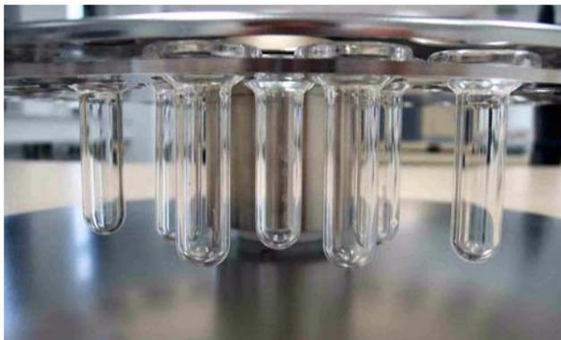
**Figure 2-36.** Turret and Correct Vertical Placement of Vials
