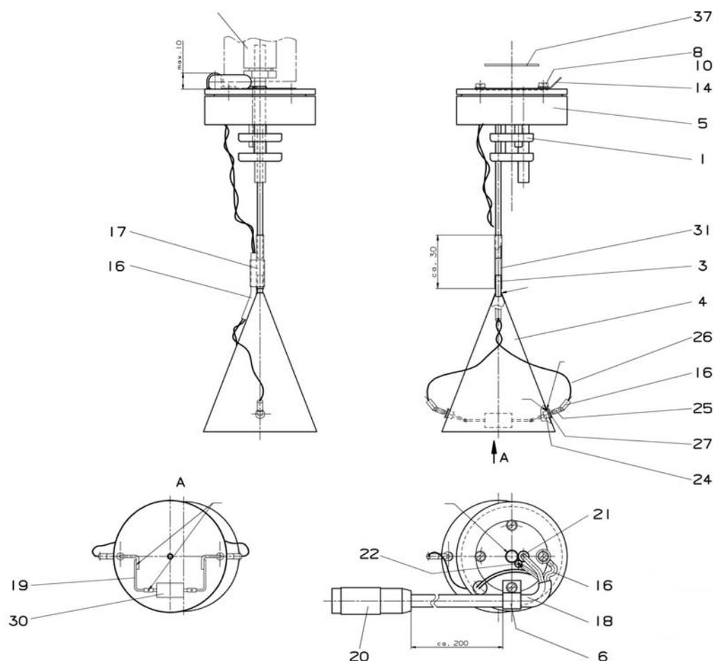
**Figure 6-21.** Cooling Unit (Part No. 079 2400)\*
