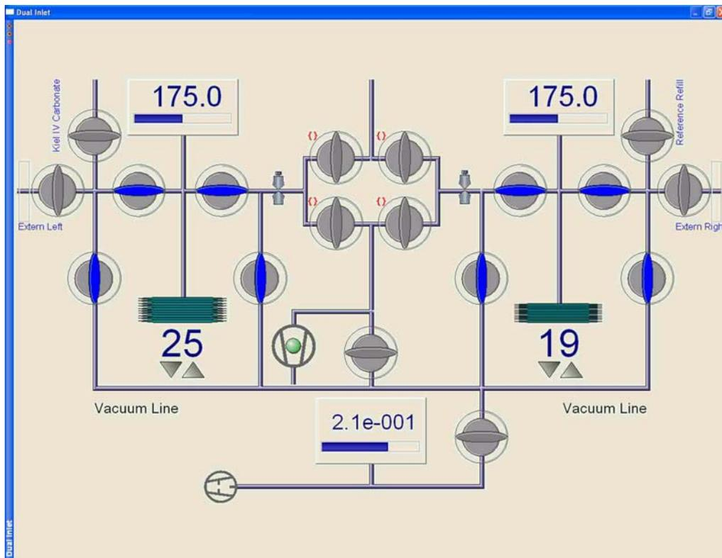
**Figure 4-7.** Matching Sample Capillary to Standard Capillary
