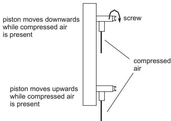
**Figure 2-39.** Piston Speed Adjustment
