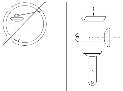
**Figure 5-4.** Correct Sample Placement
