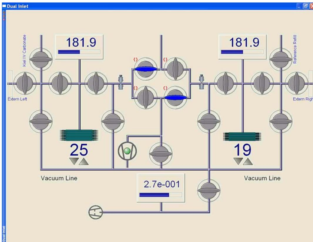
**Figure 6-31.** Leak Check of Pneumatic Valves - Step 6
