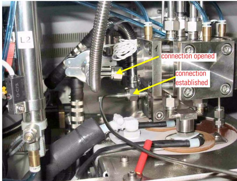
**Figure 4-10.** Connecting Transfer Tube to Kiel IV Carbonate Device
