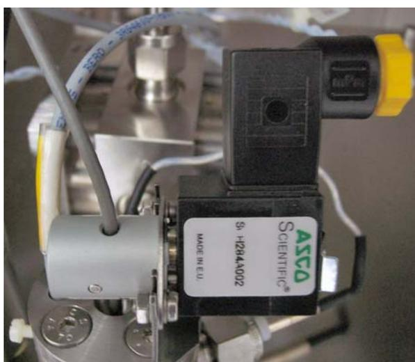
**Figure 2-63.** Mounting Pinch Valve upon Acid Valve
