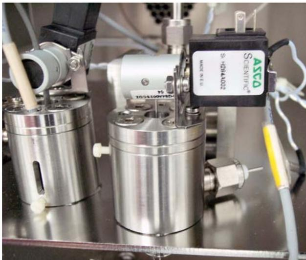
Figure 4-14. Acid Valve in Position
