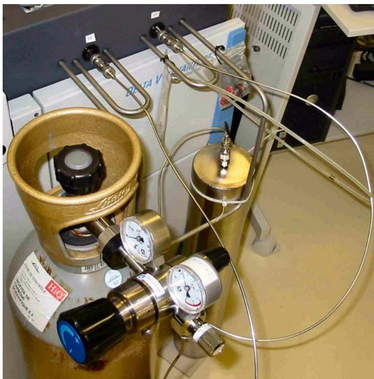
**Figure 2-55.** Filling Reference Refill Device from External Source - I
