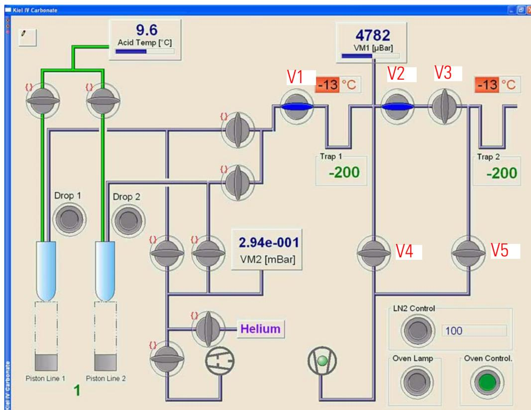
Figure 6-30. Leak Check of Pneumatic Valves - Step 5
