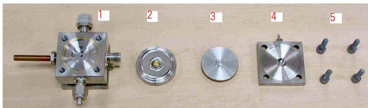
**Figure 2-24.** Parts of Dual Inlet System Valve
