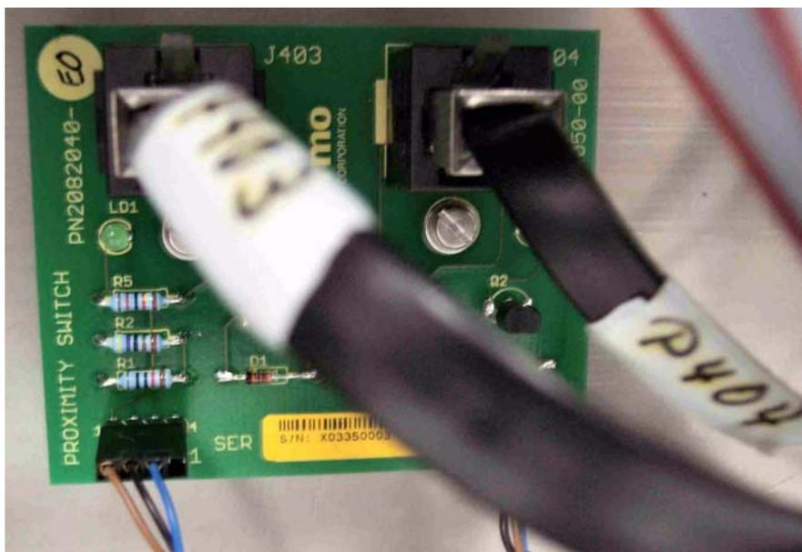
**Figure 2-12.** Interface Proximity Switches - Inlet Control Board
