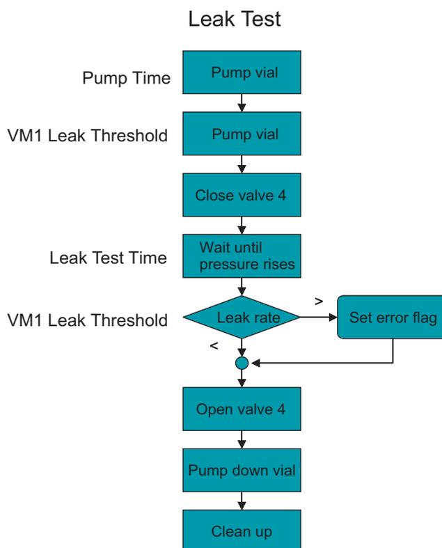
Figure 5-6. Leak Test
