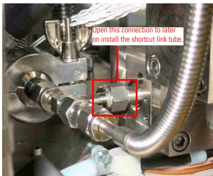
**Figure 4-9.** Connection for Installation of Shortcut Link Tube
