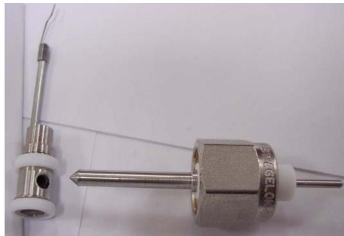
**Figure 4-17.** Drop Counter and Electrical Feedthrough
