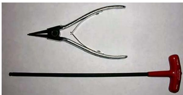
**Figure 6-25.** Tools for Valve Replacement
