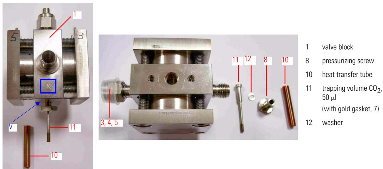
**Figure 2-29.** Microvolume and its Parts\*
