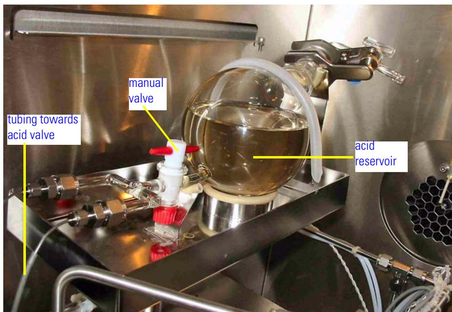
**Figure 2-58.** Acid Reservoir and Manual Valve
