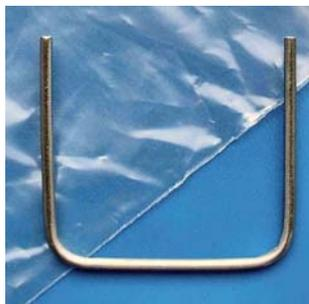
In case the position sensor shown in Figure 2-43 has eventually shifted, use the tool (Part No. 115 7390) to readjust its position.
