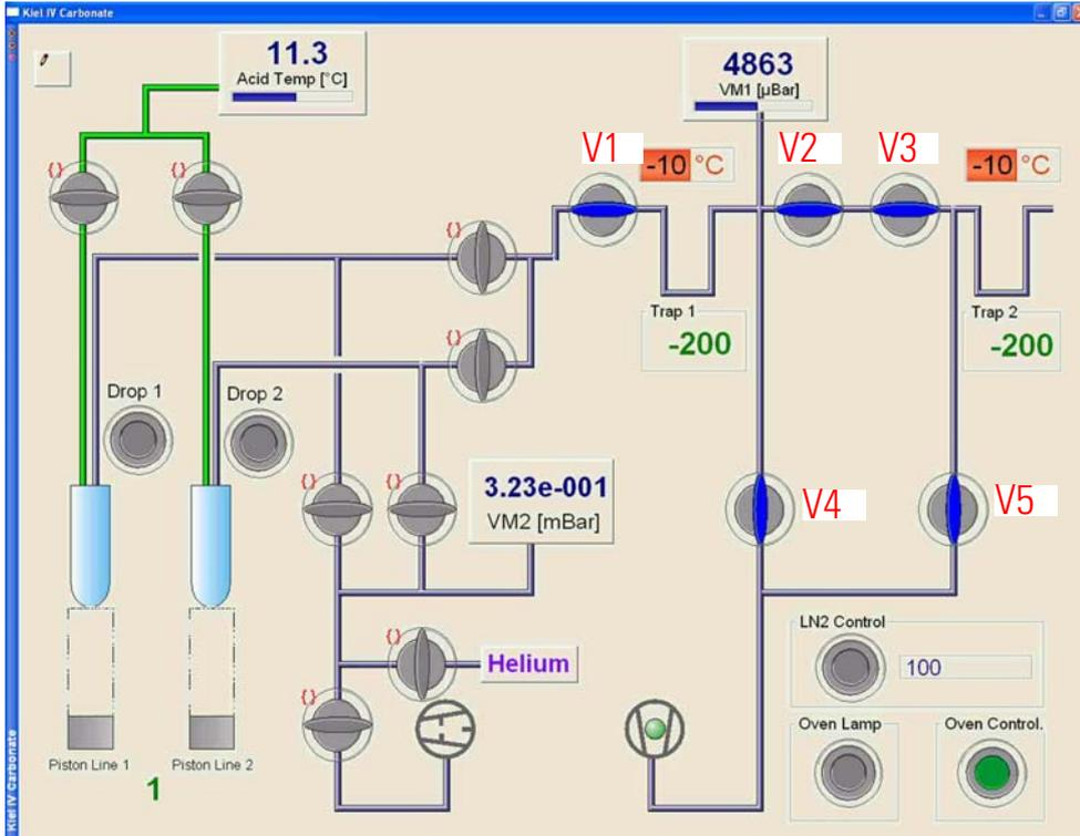
**Figure 6-28.** Leak Check of Pneumatic Valves - Step 1
