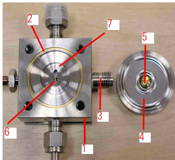
The stainless steel membrane 4 is turned down by 180° and then laid onto the gold-made gasket 2, that is with the plunger 5 oriented downwards.
