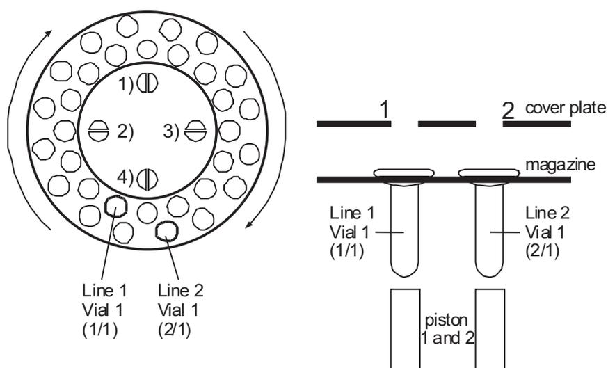
**Figure 2-38.** Magazine with Cover Plate and Vials
