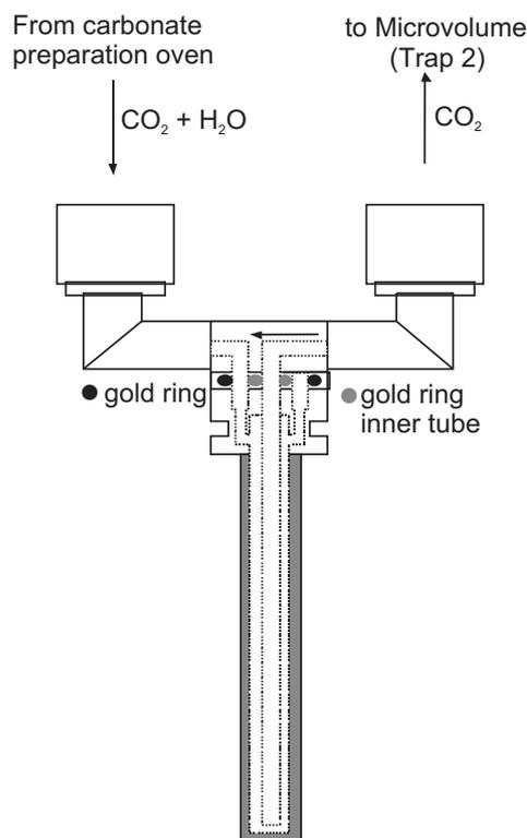
**Figure 2-28.** Schematic of Trap 1\*
