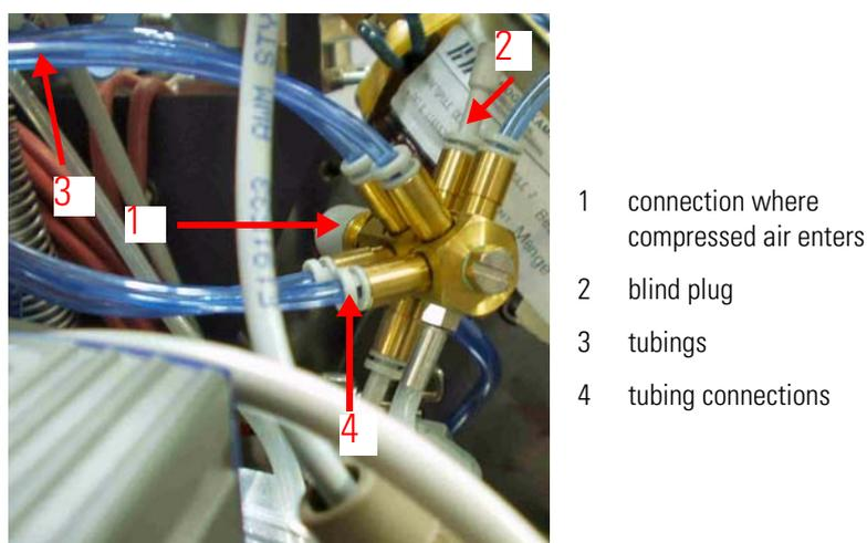
**Figure 2-27.** Compressed Air Distributor
