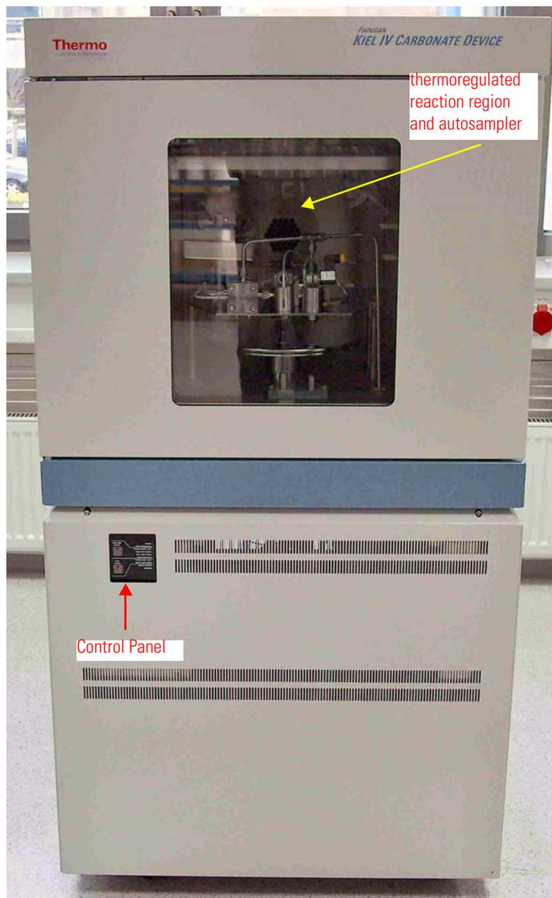
**Figure 2-1.** Finnigan Kiel IV Carbonate Device - Front View
