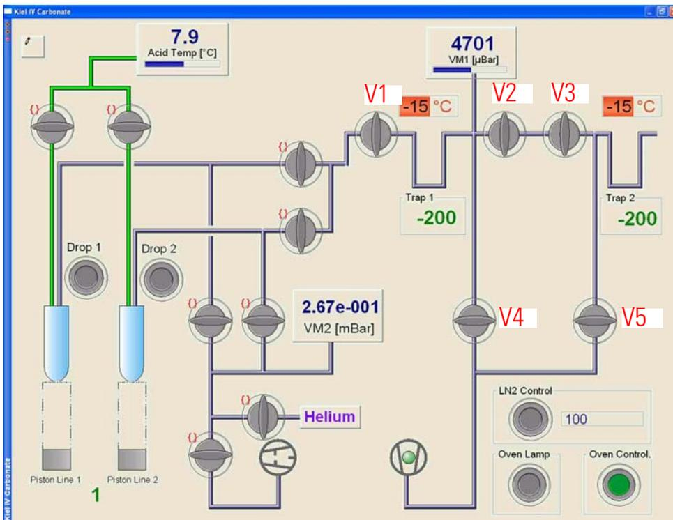
**Figure 6-29.** Leak Check of Pneumatic Valves - Step 2
