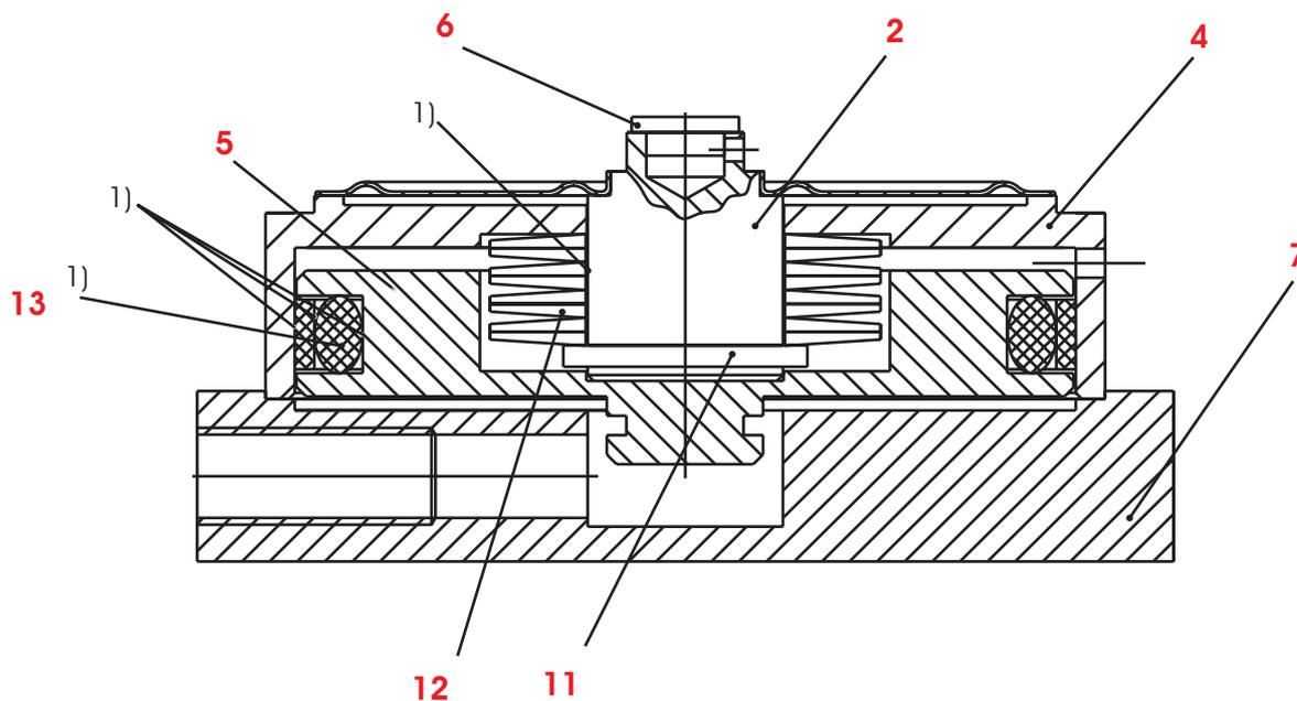
**Figure 6-24.** Valve Unit (Part No. 065 3001)\*
