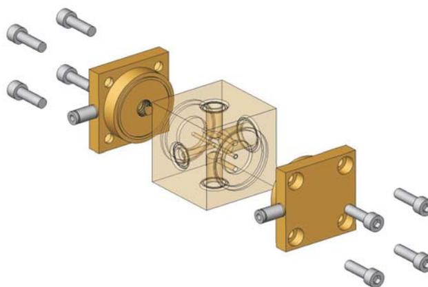
Figure 2-25. Double Valve Block
