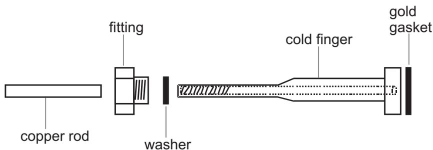
**Figure 2-30.** Microvolume Parts to be Inserted into Autocool Unit
