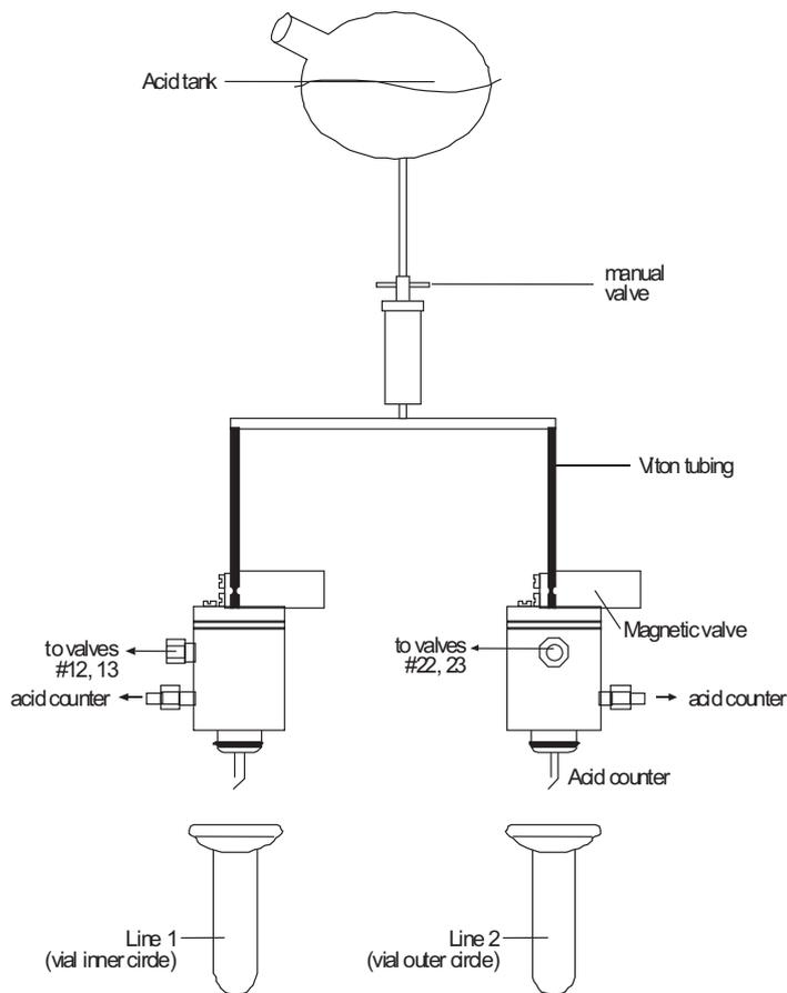
**Figure 2-57.** Schematic of Acid Flow
