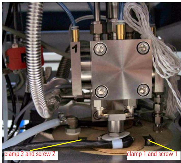
**Figure 2-33.** Mounting Instructions for Autocool Unit onto Trap 1
