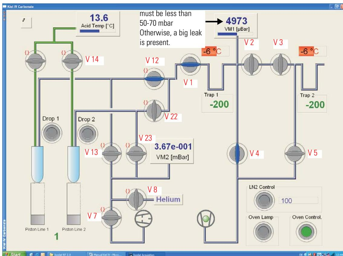
Figure 6-27. Checking VM1 Pressure Increase of Line 1
