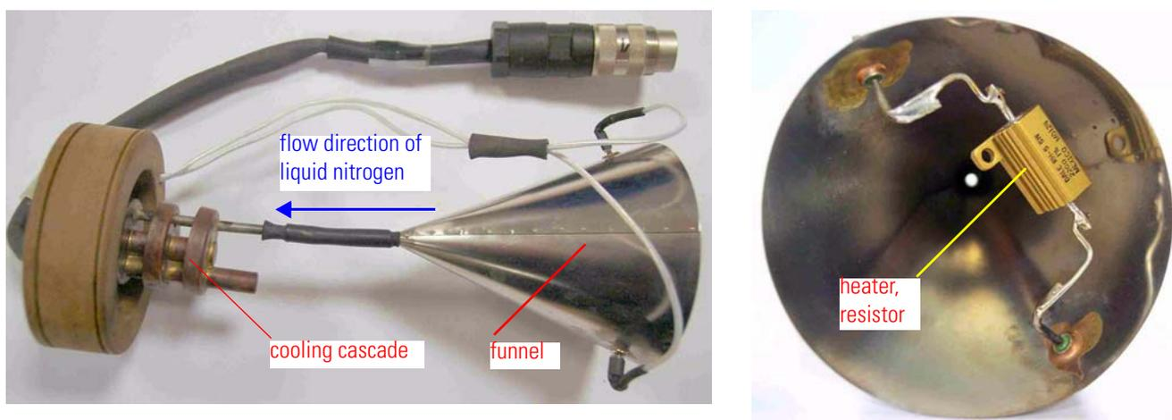
**Figure 2-31.** Autocool Unit and Interior of Funnel
