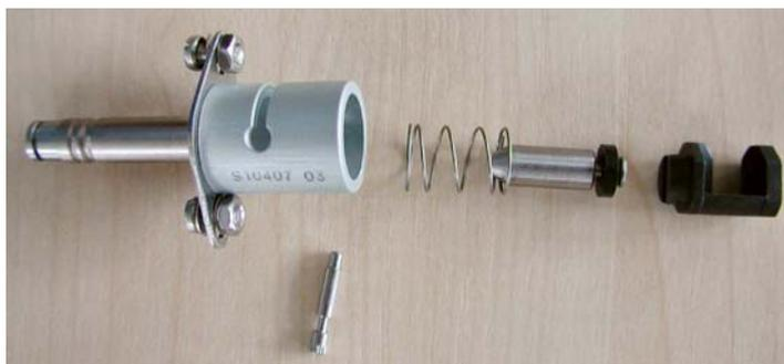
**Figure 2-61.** Pinch Valve - Disassembled
