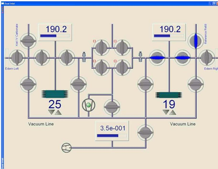
**Figure 5-18.** Reference Refill Process - Step 3
