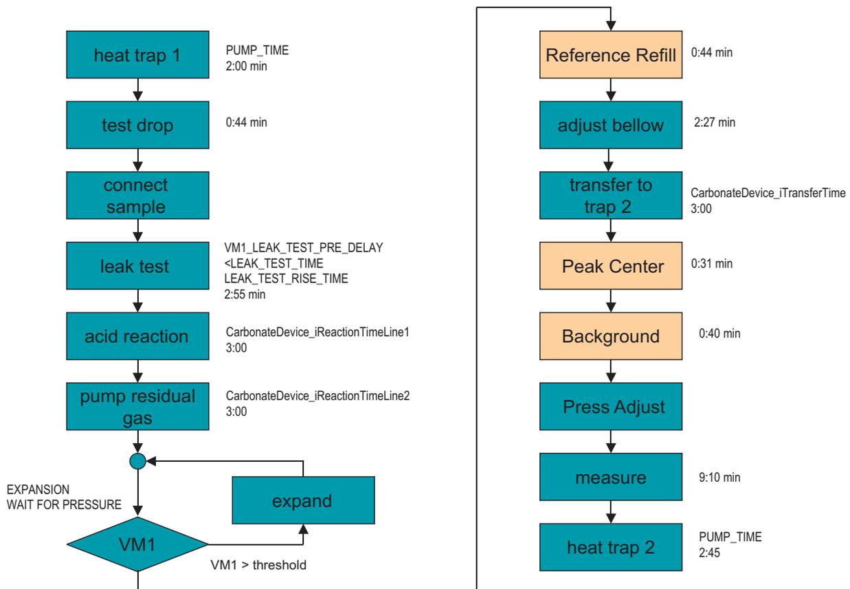
**Figure 5-5.** Flowchart of Carbonate Process Including Timing
