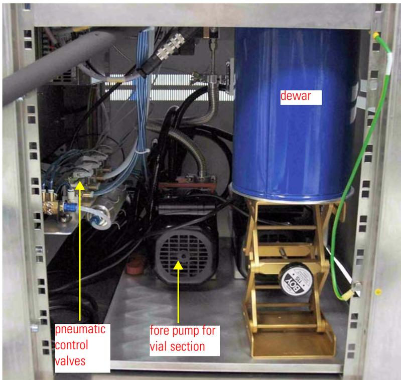
Figure 2-5. Front Panel - Lower Part
