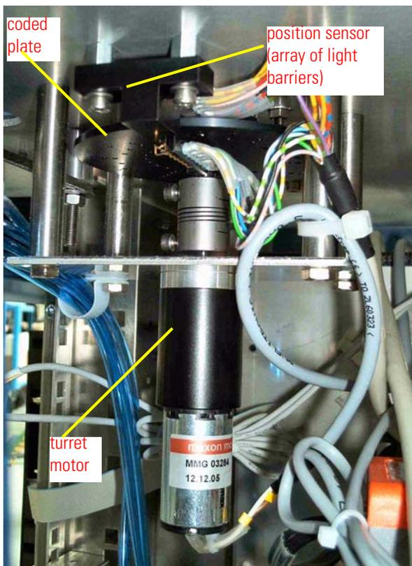
Figure 2-43. Turret Motor and Position Sensing Array
