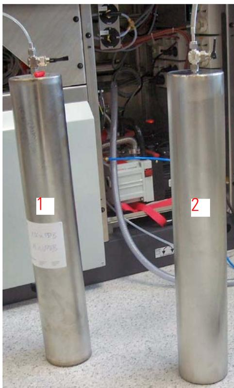
**Figure 2-53.** Reference Gas Refill Units
