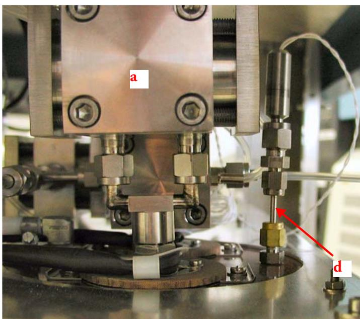
**Figure 2-4.** Close-Up View of Trap 1 and Sensor for Fill Level
