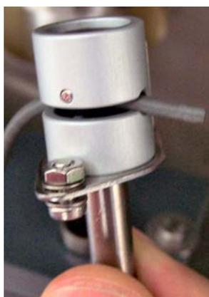
**Figure 2-62.** Feeding Acid Tubing into Pinch Valve
