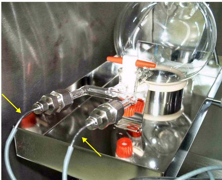
**Figure 2-16.** Connecting Viton Tubes of Acid Valves
