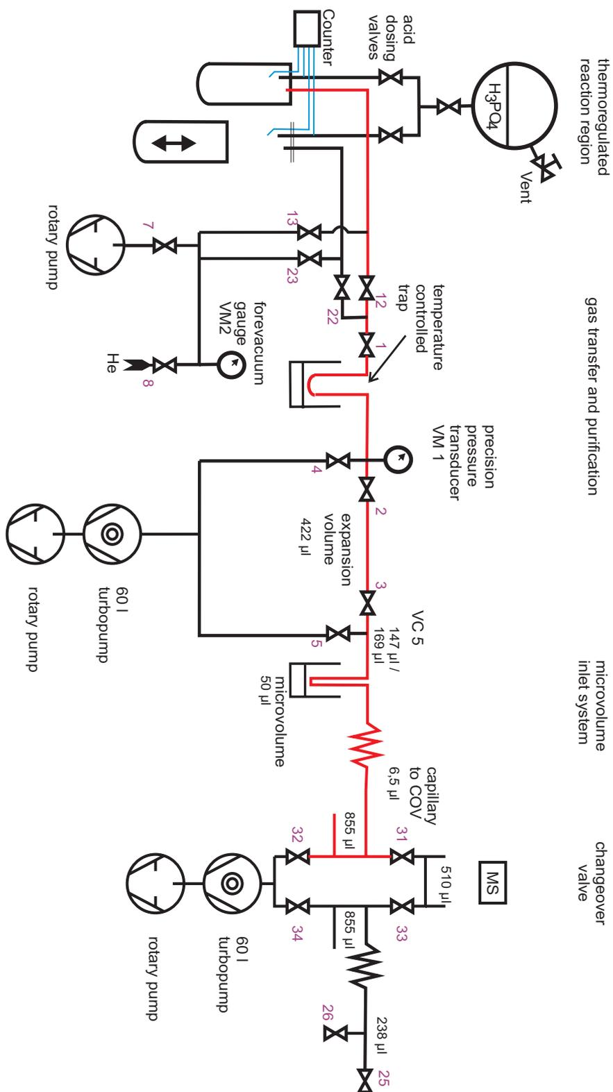
**Figure 6-42.** Kiel IV Carbonate Device - Vacuum Schematic
