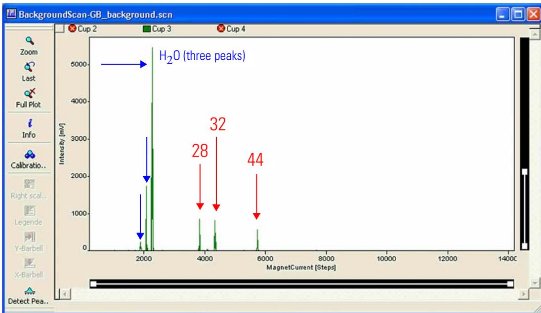
Figure 4-2. Mass Spectrum of Background Gas Composition \*
