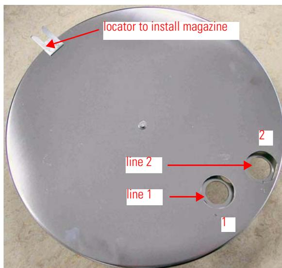
**Figure 2-37.** Turret and Lid for Line 1 and Line 2 Position
