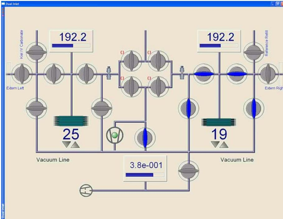
Figure 5-16. Reference Refill Process - Step 1
