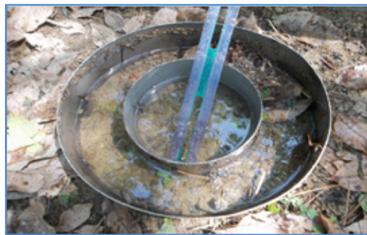
Figure 1. Measurement of soil water infiltration with a double-ring infiltrometer.
