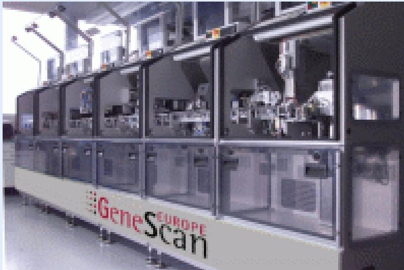
Fully automated microarray production system based on TopSpot technology (TopSpot /P) and operated at GeneScan Europe AG
